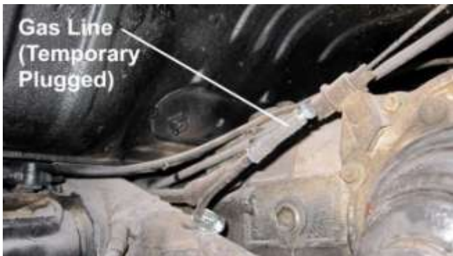
1663. A close up view of the gas line shown temporary plugged.
