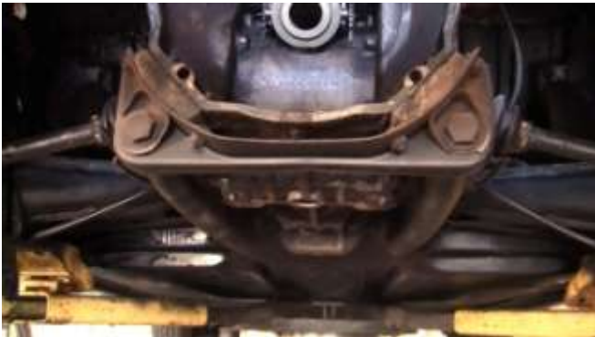
1658. View of the transmission support brackets.
