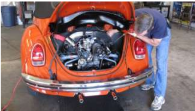
1683. Tommy connecting the two top bolts.
