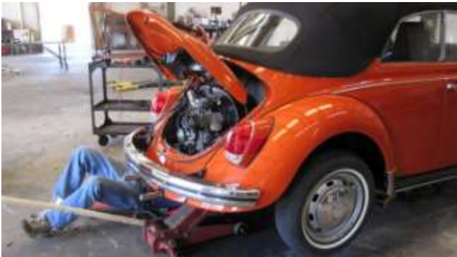
1682. Tommy connecting the two bottom bolts, gas line, and heater cables.
