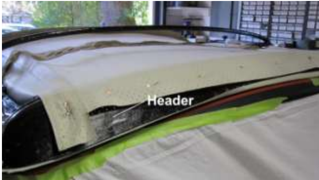
1345. The headliner was pulled uniformly and a first row of tacks were installed on the header (4).
