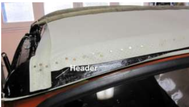
1347. The header (4) after the second row of tacks have been installed.
