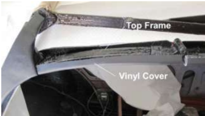
1356. Frame side shown with vinyl cover attached.
