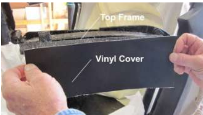
1355. Slowly apply the vinyl covering to the frame and rub out any air pockets.
