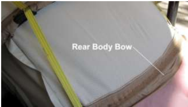
1344. The rear body bow (3) after attachment.
