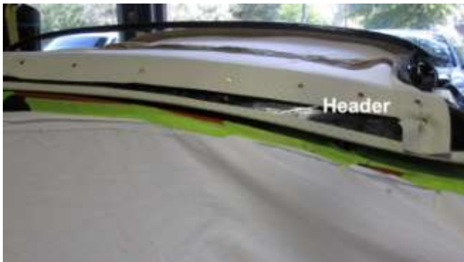
1346. The header (4) after the first row of tacks have been installed.
