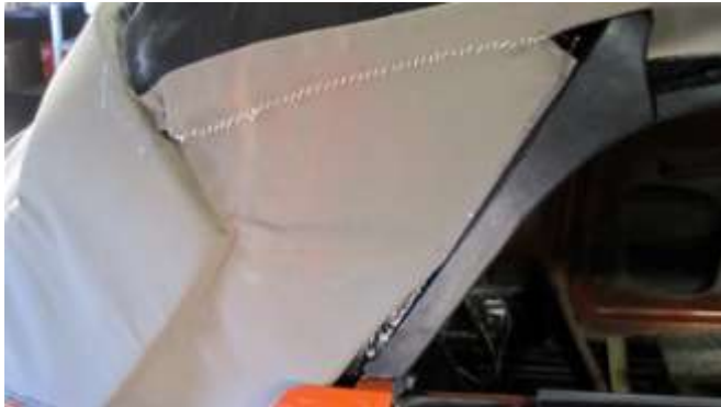
1377. The right side panel shown after sewing to the top panel.
