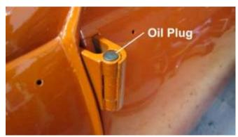
1109. Install the new oil plugs on each door hinge.
