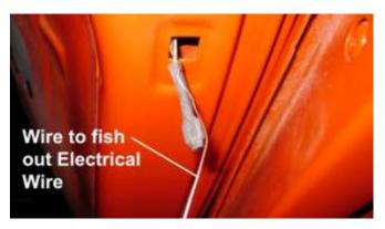
1141. With a steel wire, fish the door switch wire out for the passenger or right side of the car.
