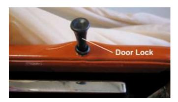
1110. Install the door lock buttons on each door.
