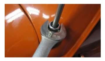
1132. Attach the aerial flange and nut and tighten with a 17mm wrench.
