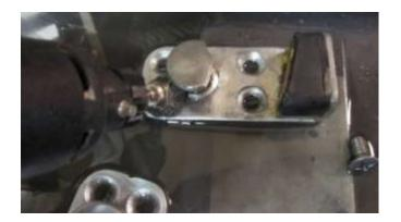
1104. Clean up the door striker plates with a hand grinder using a wire brush and WD-40.
