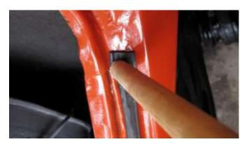
1126. Also bend the body seam down on the rubber seal at the ends.
