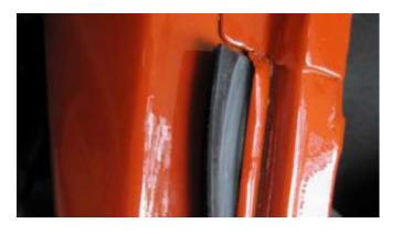
1123. Start on the deck lid seal at one of the corners and slide it into the body seam.
