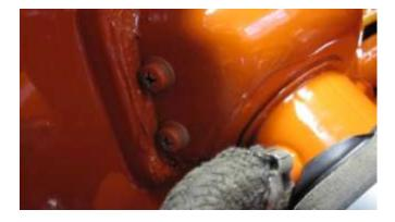
1111. Install the two screws to the gas tank filler door from the trunk. Check to make sure the gas tank filler door open properly.
