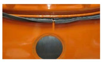
1121. Cut the extra length of seal at the bottom using a pair of scissors and add a wire clip to hold the seam together.
