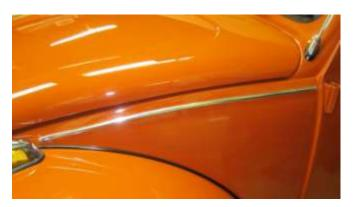
1162. Snap the side molding onto the body clips.
