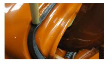
1119. Use a hammer and wood dowel to push the seal down at the rubber pins on the opposite side. Bend the body seam down slightly at the ends.
