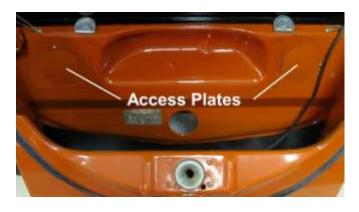
1139. With sheet metal screws attach the two access plates as shown. Do not attach the center access plate at this time.
