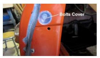
1155. Install both clear plastic bolt hole covers on the door frame and door jams.
