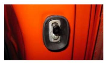
1144. The door switch and new rubber gasket installed on the passenger or right side.
