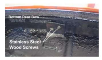
1152. Connect the bottom rear bow to the flange on the body with stainless steel wood screws in three locations.
