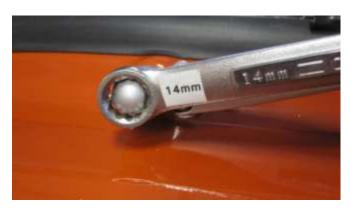
1134. Insert the plastic windshield cover, then the windshield wiper and tighten the nut with a 14mm wrench, as shown.
