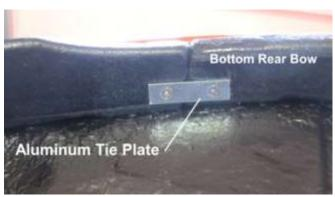
1153. Since the new bottom rear bow was in three pieces I added the aluminum tie plate as shown with stainless steel wood screws to tie the three pieces together to make the bow more rigid.
