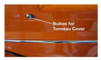
1164. Install the button for the tonneau cover tie down.
