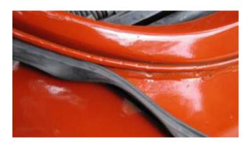
1124. Slowly insert the new seal in the body seam around the engine opening.
