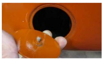
1137. Install the access hole plug from the outside of the body. This is the access hole to pull the gearshift rod out of the car if needed.
