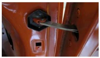
1113. Install the door check rods with new seals, as shown.
