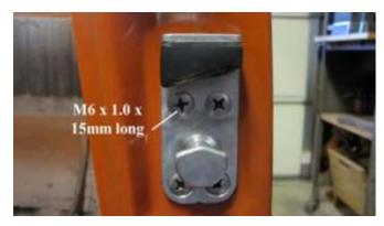
1105. Install both door striker plates on the VW body with screws, as shown.
