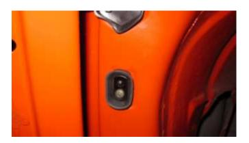
1146. The door switch and new rubber gasket shown installed on the drivers or left side
