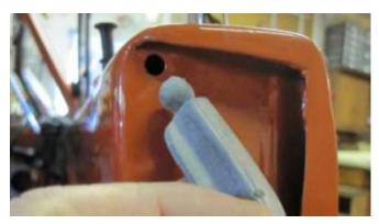
1147. Install the new door seal by starting at the door end, as shown, and with a small screwdriver insert the round portion of the seal through the round hole in the door end.
