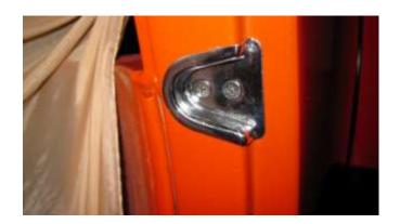
1158. Install the door alignment plate on the body.
