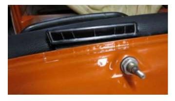
1115. Install the new fresh air vents, as shown.
