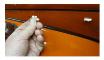
1160. Install the molding clips in the body holes, as shown.
