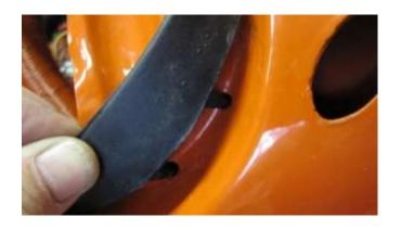
1116. Install the new hood seal by starting at the front and inserting the 3 rubber pins into the body holes. Slowly insert the seal in the opening and move to the other corner and attach the rubber pins. Note from underneath you will be able to pull one of the rubber pins through with a pair of pliers, but the other two you will have to push through.
