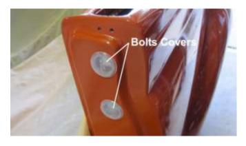
1156. All together there are 12 clear plastic bolt hole covers to be installed on the door frame and door jams.
