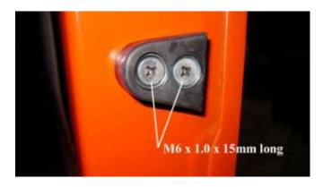
1108. Install the new door alignment plates on both doors.
