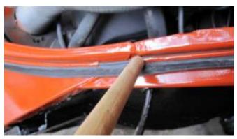
1125. With a hammer and a wooden dowel bend the body seam down onto the rubber seal at the corners.
