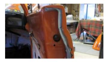
1148. Test fit the seal all the way around the door side. Then pull the seal out and insert 3M adhesive on the door and push the seal back into the slot.
