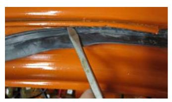
1118. Use a small screwdriver to insert the seal into the body seam. Be careful and do not let the screwdriver slip off the seal messing up the new paint job.
