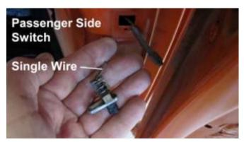
1142. The passenger or right side door switch only has a single wire as shown in the diagram below.
