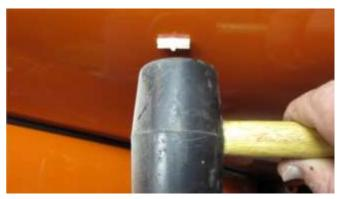
1161. Carefully tap the small plastic pin in, to tighten the clip on the inside of the body. Use a rubber mallet to protect the paint job.
