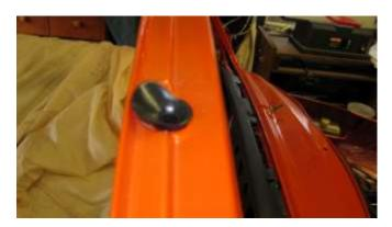
1114. Install the new grommet for the convertible top pin, as shown.
