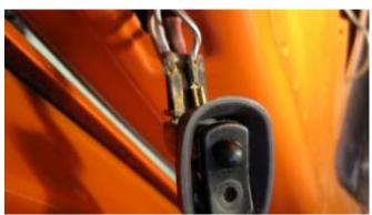
1145. Connect the four wires to the driver (left) side door switch according to the wiring diagram on the previous page.
