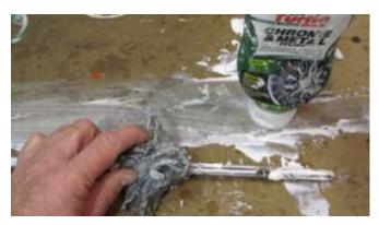
1159. Clean the chrome side molding with steel wool, chrome and metal polish to a nice shine in preparation for installation.
