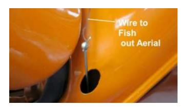
1131. Insert the radio aerial into the trunk and attach a small wire to fish it out of the opening.
