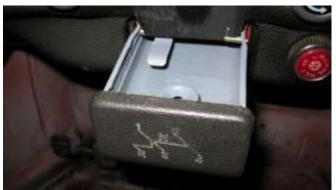
1130. Insert the ash tray into the ash tray compartment on the dash.
