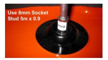
1138. From inside of the tire well, attached the access hole back plate as shown with a 8mm socket.
