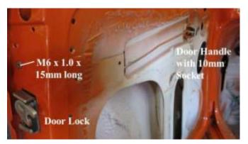
1106. Install the door lock assembly and door handle on each door with screws, as shown.
