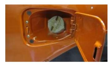
1112. Install the new gas tank door rubber bumpers, as shown.
