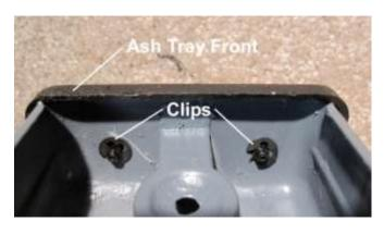
1129. Attach the ash tray front to the ash tray body with the metal clips.
