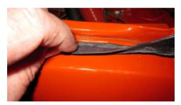
1117. Attach the hood seal in the body seam along the top.
