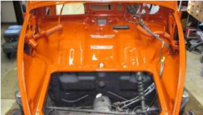
835. Topcoat completed with a coat of prime sealer and 2 coats of Nason Dupont Nason Urethane. The mix ratio is the same as the previous urethane Clementine paint, 8:1:2.
