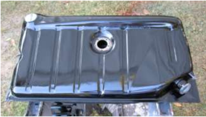
839. The gas tank with the topcoat completed. No Flatter was used on the mix for the tank since the original color was a gloss black.
