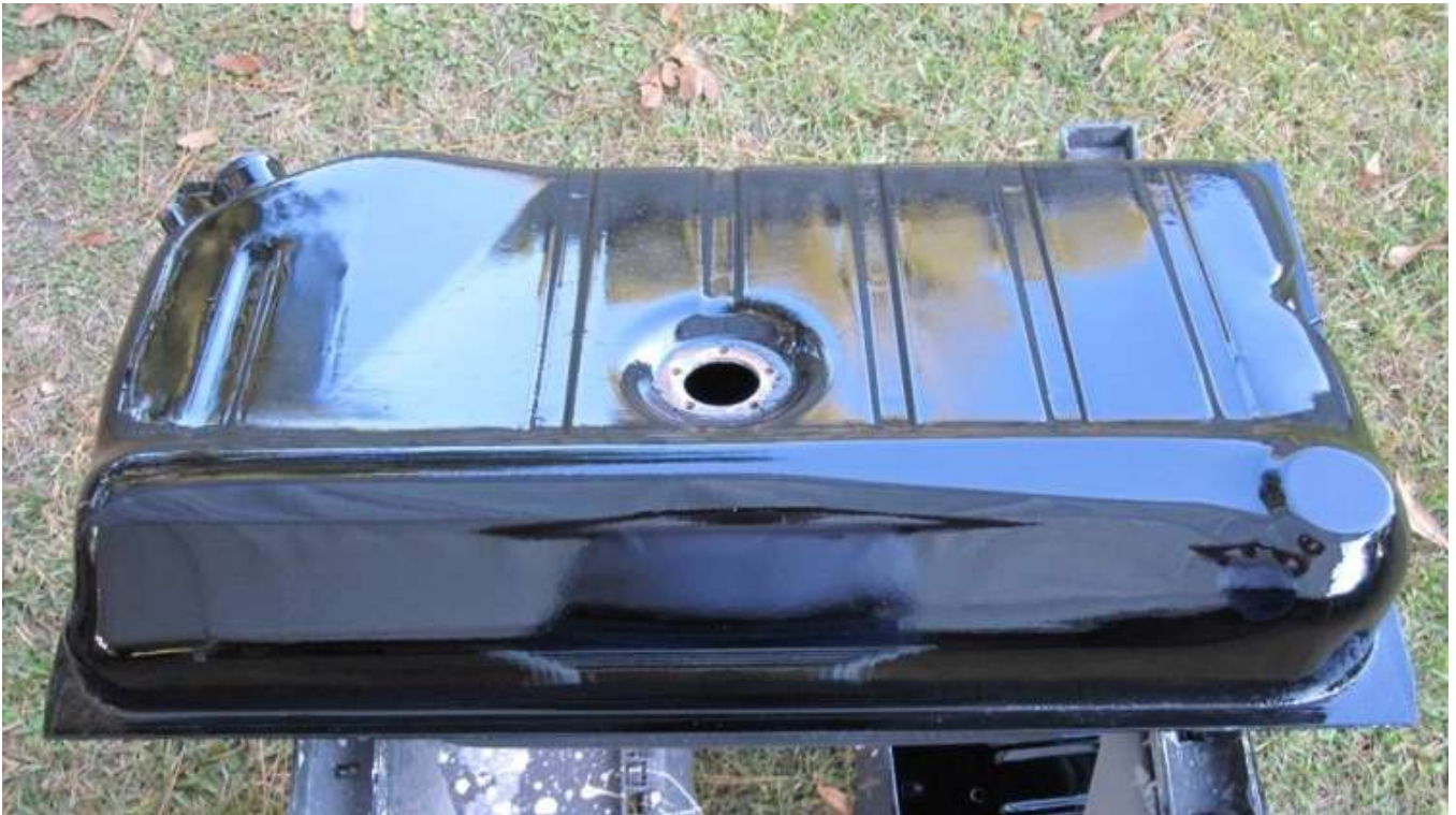
840. The gas tank after two coats of Dupont Nason Urethane black paint. The mix ratio is the same as the previous urethane Clementine paint, 8:1:2.
