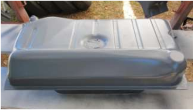
838. The gas tank after one coat of prime sealer.
