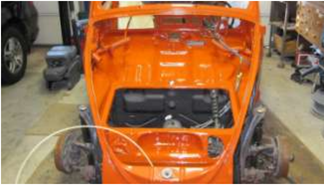
834. Finished topcoat on trunk interior.
