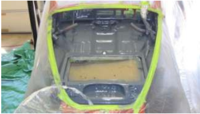
830. One coat of prime sealer completed.
