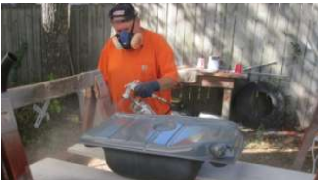
837. Vic Diabin, spraying the prime sealer, on the gas tank.
