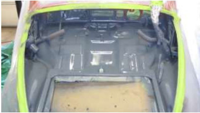
831. Close up of prime sealer.
