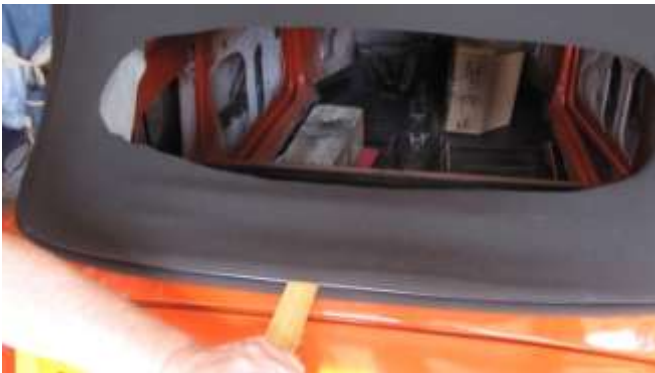
1422. Next cut slits in the corners of the rear window, to allow the top cover to fold over and staple.
