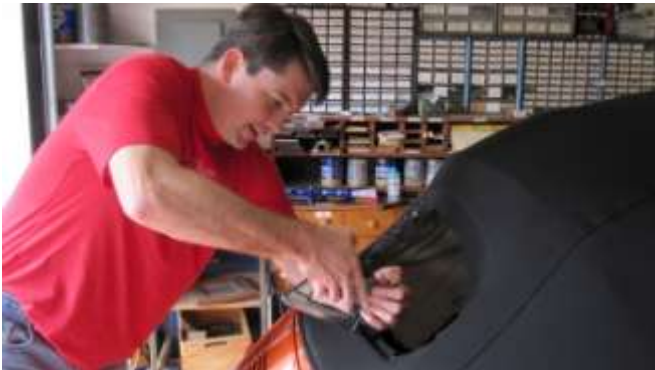
1423. My son, Neil Beasley stapling the top cover to the interior wood frame.
