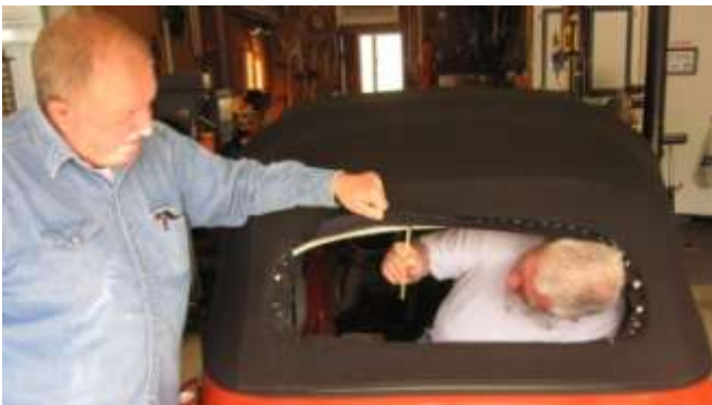
1424. Vic holding the top cover up, so I could spread glue on the underside of the top and on the exposed edge of the frame.
