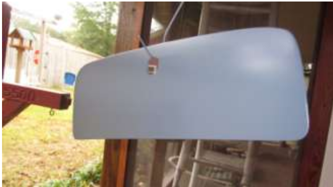
1248. Pocket door painted with prime sealer.
