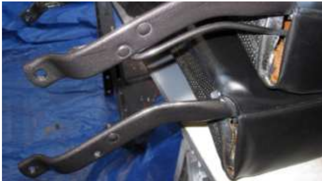
1252. Seat back support arm painted with the finish coat.
