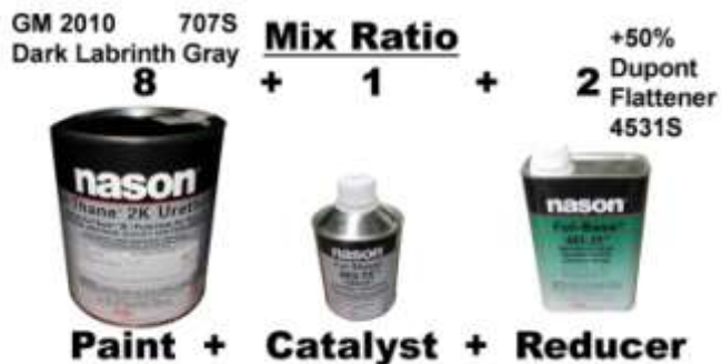
1249. I used the same type of Dupont Urethane used to paint the car. The paint store could not determine the proper mix for the original color seat color (L43 grey-black) so I used my pocket door to pick the closest paint I could find which was a General Motors 2008, 2009 & 2010 707S dark labrinth gray. As shown, I added 50% of Dupont flattener to make it more of a satin finish. In hind sight the finish still had too much gloss, so 75% would be better.
