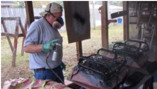
1251. Vic Diabin painting the finish coat on the seat bottom frames.
