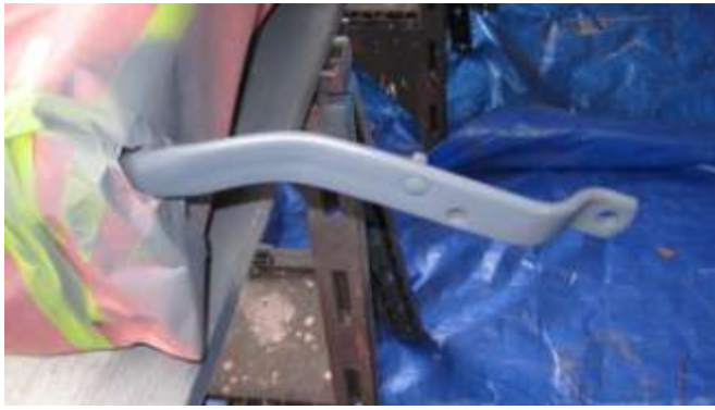
1246. Seat back support arm painted with prime sealer.
