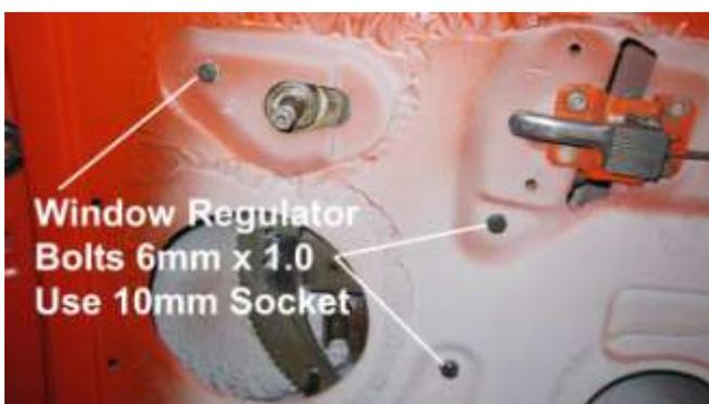
1052. The window regulator is connected with 3 bolts, as shown.
