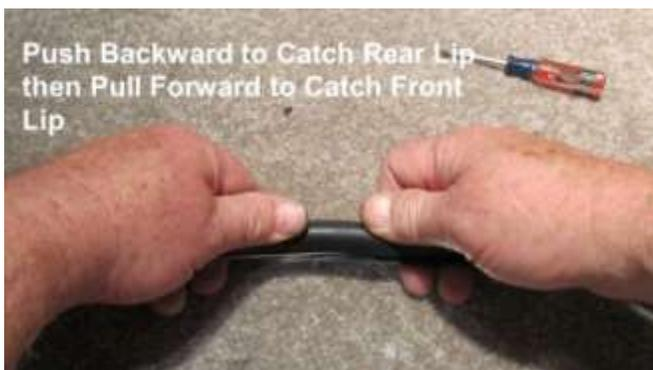
1080. Push the seal backward to catch the rear lip on the glass, then pull the seal forward to catch the front lip, then push down. Go an inch or two at a time, this can be time consuming but also very important, so do it right.
