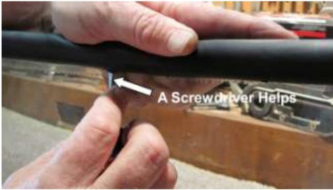
1081. Use a small screwdriver to help pull the lip out over the glass, but be careful, do not scratch the glass, penetrate your palm, or break through the window seal.
