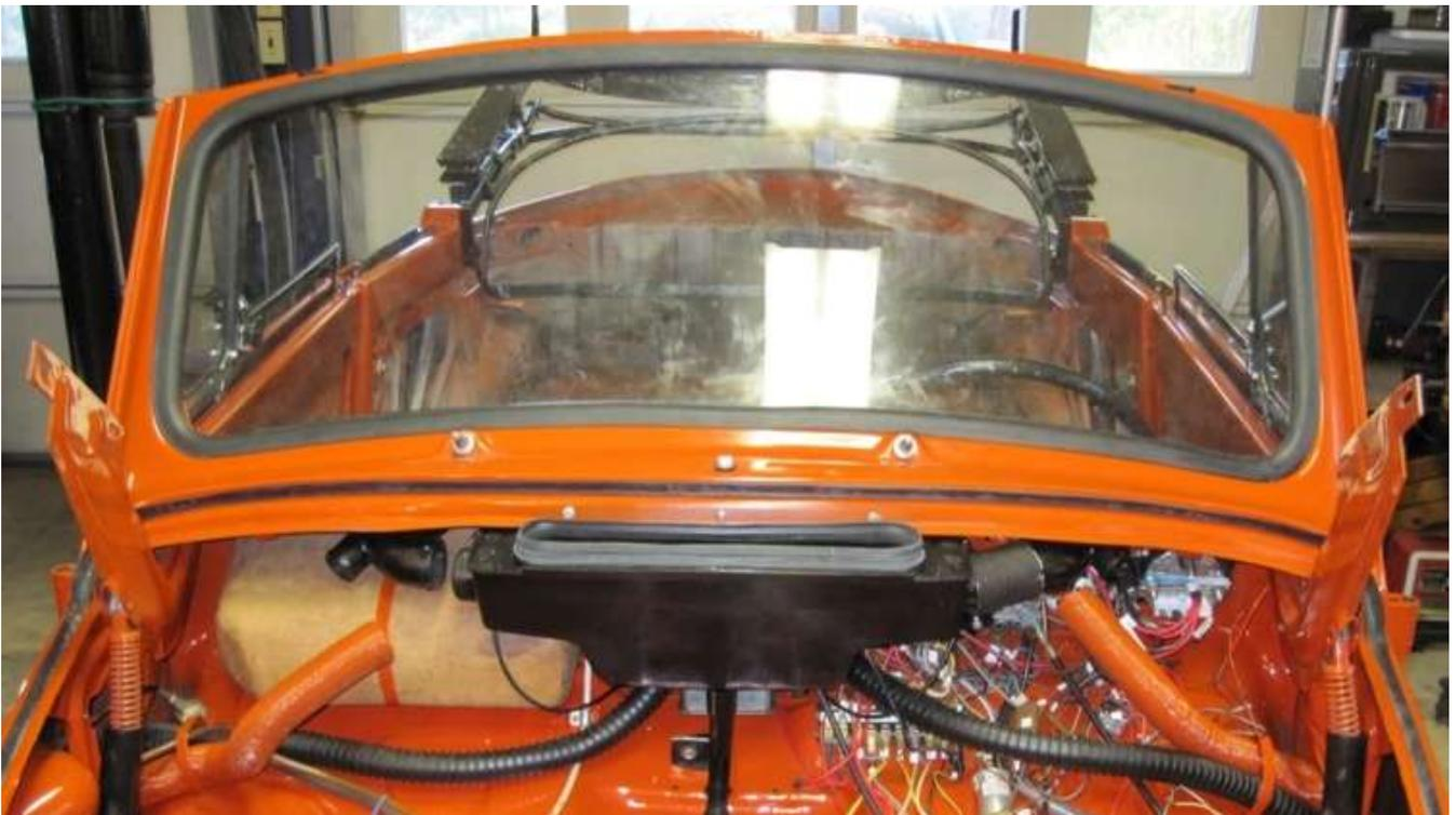
1095. All side glass and the front windshield is now installed. The back glass will be put in after the convertible top has been installed.
