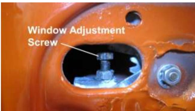
1047. From the back seat, inside the car, adjust the rear windows stop.
