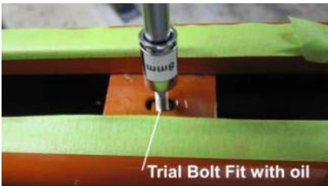
1056. Add tape to protect the car paint. Check to make sure that the nut has not fallen out on the vent window connection. Trial fit a 5mm x 0.90 bolt coated with oil to loosen any paint that may hinder the bolt insertion.
