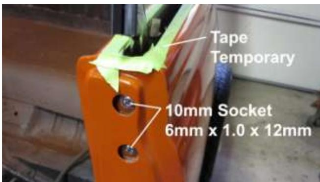
1042. Add tape as shown to protect the newly painted surface as you insert the rear window. To secure the window re-install the 2 bolts as shown.
