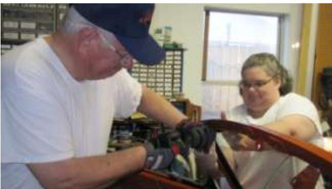
1092. Malcolm pulling line while Marcy slapping the glass and pushing in as the line creates the seal.
