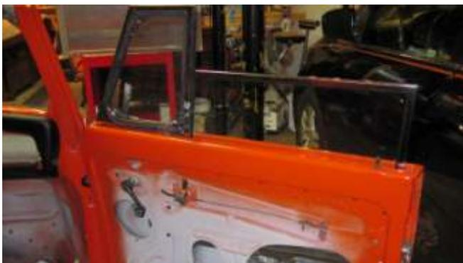
1072. Roll the window up and down several times to make the window seat in the new felt. You may need to add lubricant to the rear guide bar that rubs against the chrome window frame. Now tighten the window frame and guide bar bolts and nuts.
