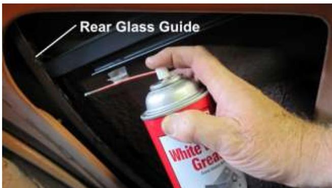
1043. Spray white lithium grease on the rear metal window guide
