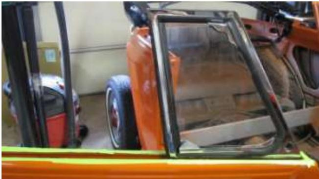
1063. A view of the vent window installed.
