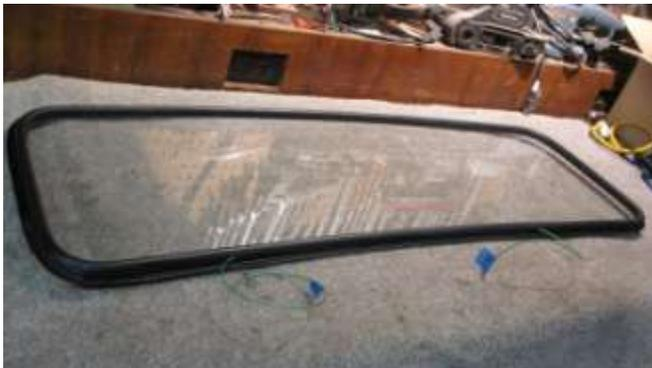
1083. The rubber seal shown installed on the front windshield and weedeater line inserted in the groove, used for installation on the car.
