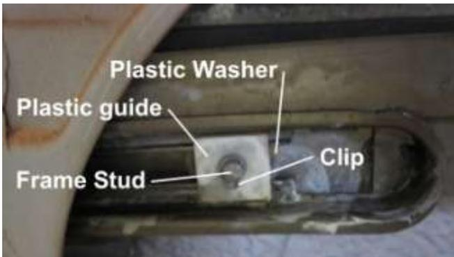
1070. Add a plastic washer to the back side of the guide bar and a plastic guide on the front side and secure with a metal clip, as shown.
