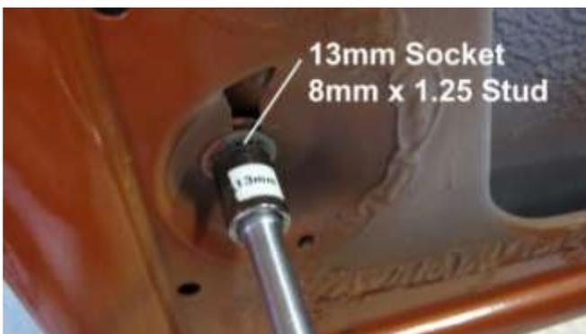
1060. With a 13mm socket connect the window glide nut near the rear bottom of the door, but do not tighten yet.
