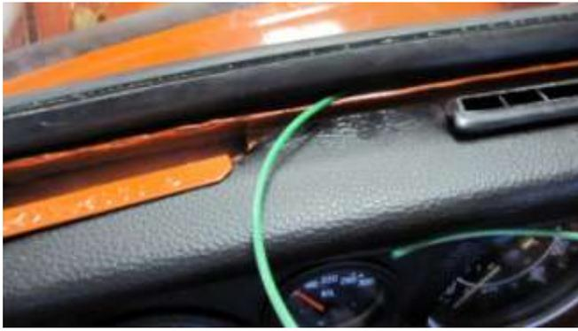
1085. Weed eater line inserted into the seal and the window glass is set in place. Window was tapped to make sure it seated into the frame.
