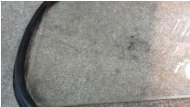
1078. Carefully, pull the seal to catch over the opposite corner, make sure not to lose first corner.
