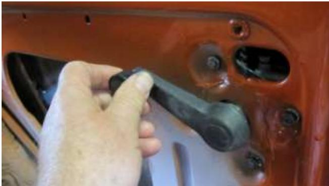
1046. Attach the window handle and raise and lower the glass several times to loosen up the movement. Add more grease and adjust the window as needed. Follow the same procedure for the opposite side rear window.
