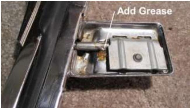
1054. Add grease to the vent window pivot arm on the vent window frame, as shown.
