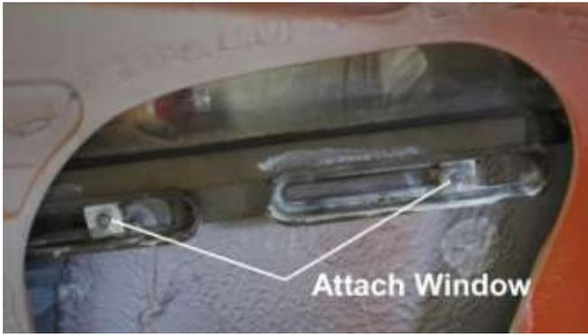
1069. Crank the window crank until the window guide bar frame and the window regulator studs are in alignment and attach window, as shown below.
