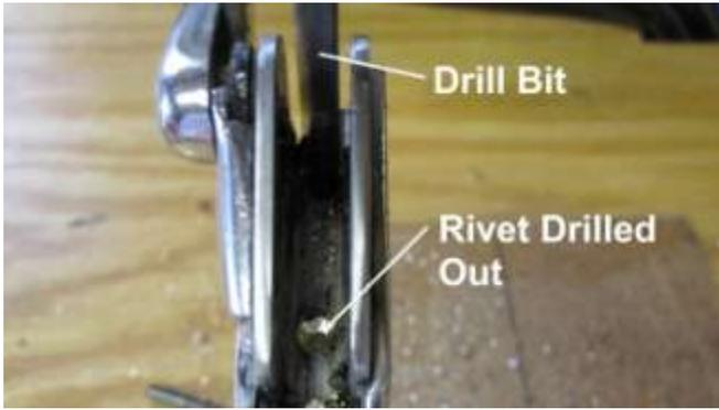
1065. Use a drill press to drill out the rivets that hold the vent window knob in place, as shown.
