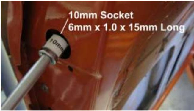
1061. With a 10mm socket connect the window guide on the end of the door frame with the 6mm nut, as shown.
