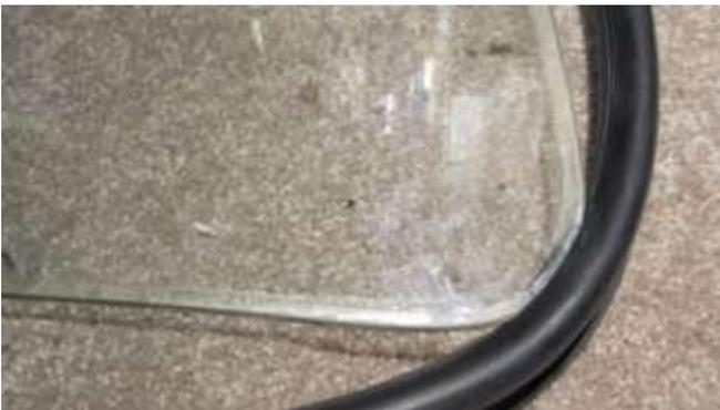
1076. Carefully, pull the seal to catch on one of the corners and hold the seal tightly against the glass.
