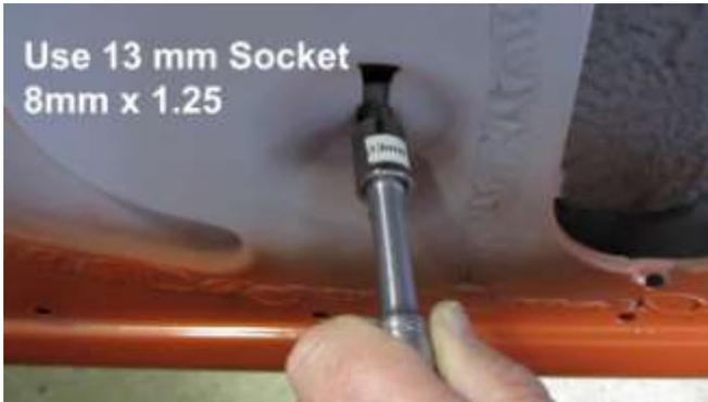
1058. Use a 12 mm socket to connect the vent frame arm from the inside, with a nut near the bottom of the door, but do not tighten yet.
