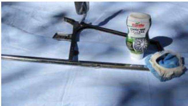
998. Clean the vent window frame with chrome polish and a fine grade steel wool. Then polish the chrome with chrome polish and a polishing rag as shown. Then buff the frame with a buffing rag.
