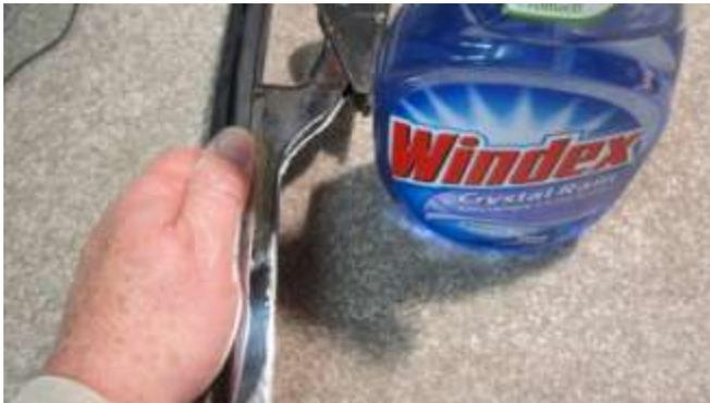
1027. The use of Windex helped the rubber molding slide onto the frame.
