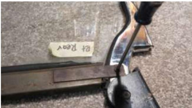
1012. With a Phillips screwdriver remove the right screw on the bottom frame and place them in a container for safe keeping.
