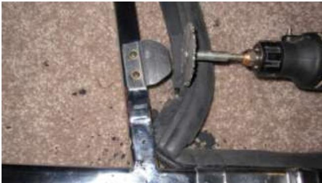
1003. To protect the bracket, put a piece of carpet on the workbench. There is one place where the rubber molding does not fit due to the rivets in the frame, as shown. Cut away the rubber in this area with a hand grinder, and install.
