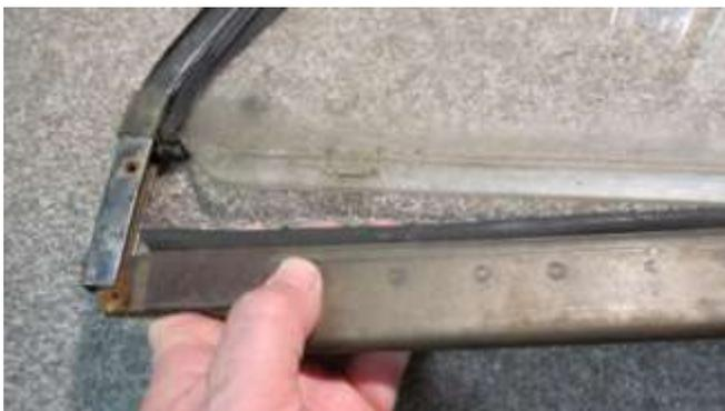
1013. Carefully pull the bottom frame out from the window.
