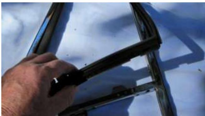
1001. Insert the new rubber vent window molding.
