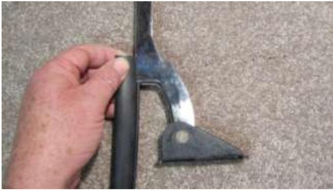
1026. Slip the new vertical end molding into the channel.
