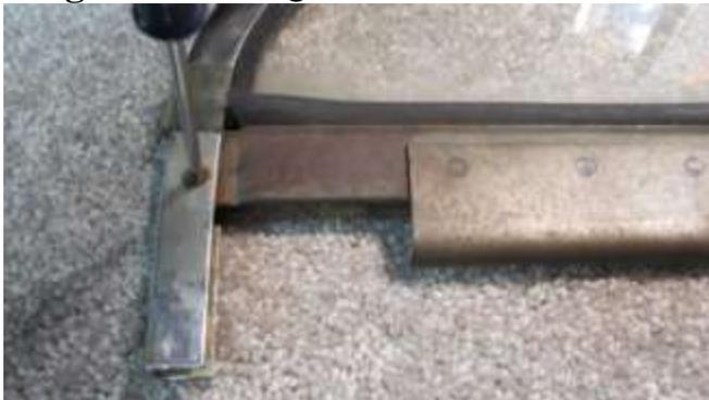
1011. With a Phillips screwdriver remove the left screw on the bottom of the frame. Place the small screws in a container to keep from misplacing them.
