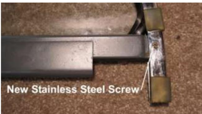
1029. Use new stainless steel screws to secure the bottom plate.
