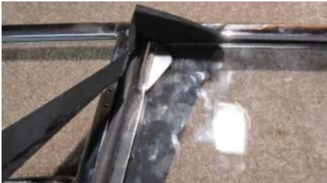
1008. Add 3M adhesive on the glass and the chrome and slide the glass into the frame.
