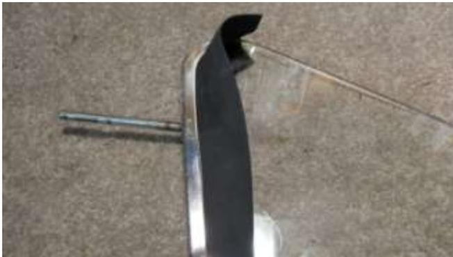
1007. The length of the molding is cut to fit, overlaps the window as shown.
