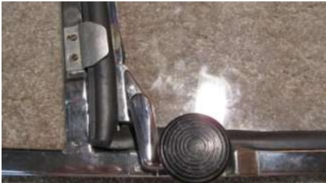
1004. The rubber molding should fit better now but, use the glass to help seat the rubber overnight.
