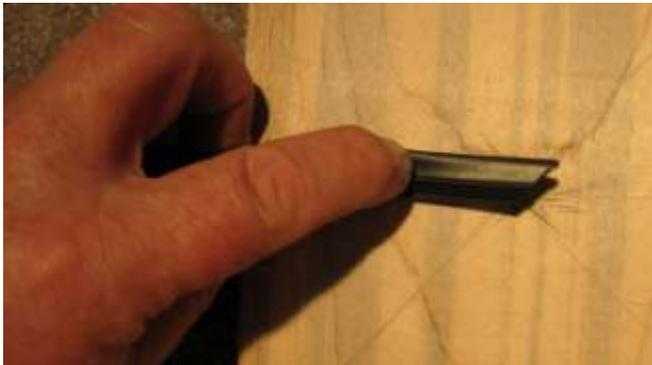
1024. Cut the window insert rubber molding to length and at a 45 degree angle where required (Using the approximate window bend is satisfactory).
