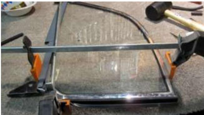
1028. Woodworking clamps were used to pull the frame together tightly so that the screws could be inserted.
