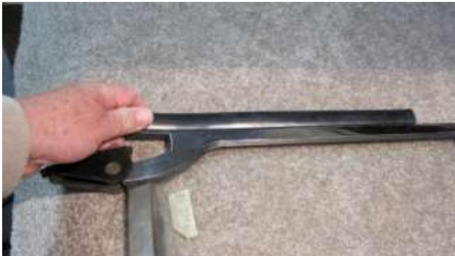
1016. Slide off the vertical end molding off the frame.
