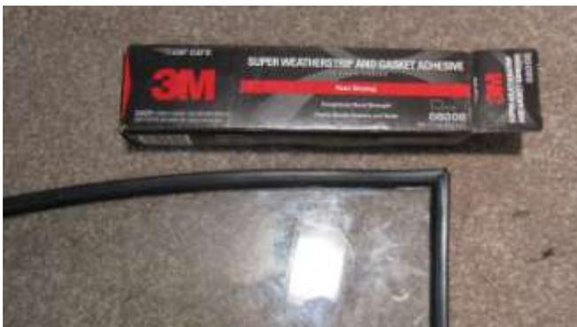
1025. I tried to install the molding and glass in the frame but the molding kept moving, so I added a little 3M adhesive to the inside of the molding and glued the molding to the glass prior to installing the unit into the frame, which worked find.
