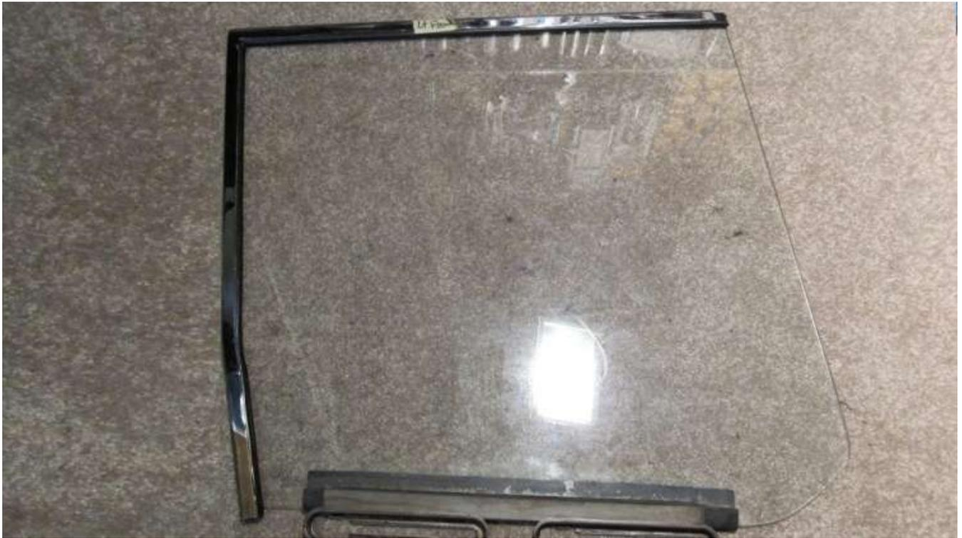
1034. Front window with the chrome metal frame attached, thanks to Kittrell Glass.
