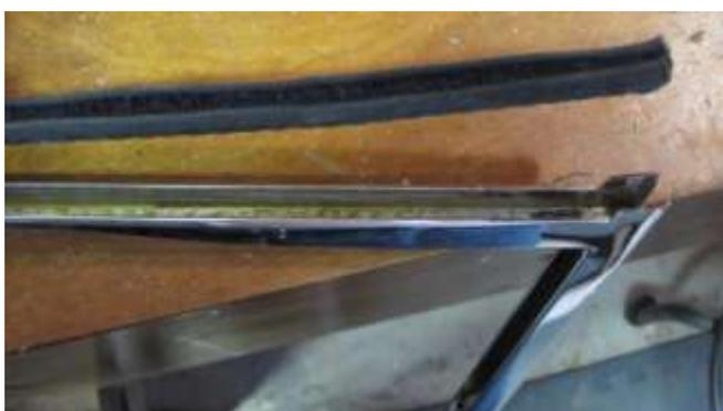
999. Pull out the window felt and replace it with a new one.
