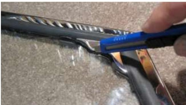
1009. Cut off the excess rubber, flush with brackets on the corner of the frame as shown.
