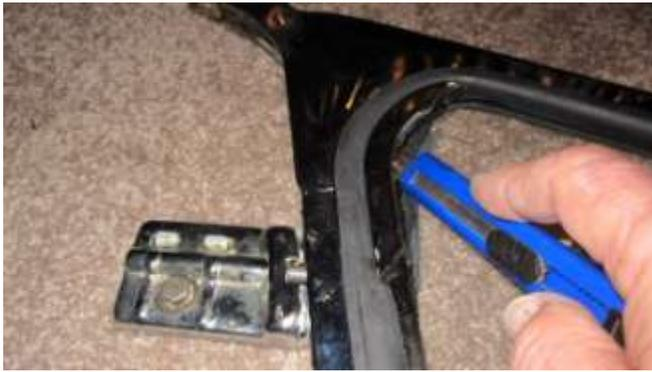
1010. Cut excess rubber around all of the chrome on the window. Put the vent glass into the frame to create a bond overnight.
