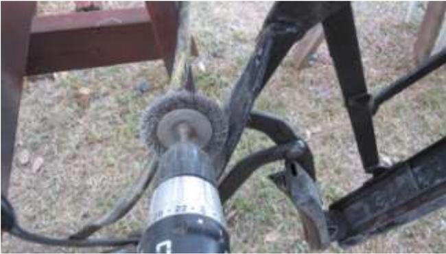
965. Move the frame outside and with a wire brush on a portable electric drill go over the entire frame assembly and remove all rust spots, flakey paint, and glue from the prior top then sand the frame with 120 grit sandpaper then with a medium grade steel wool. Remove the tacks and staples from the wood and sand both metal and wood with 220 grit sandpaper.
