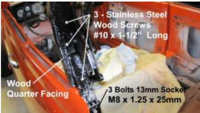
985. Place the 3 bolts, M8 x 1.25 x 25mm long, on each side of the frame to the body, but do not tighten. Then go ahead and secure the 3 stainless steel wood bolts #10 x 1-1/2" long to the wood quarter facing as shown.
