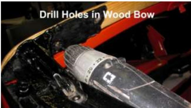
990. Drill an attachment hole for the front bow through the existing holes in the metal frame.
