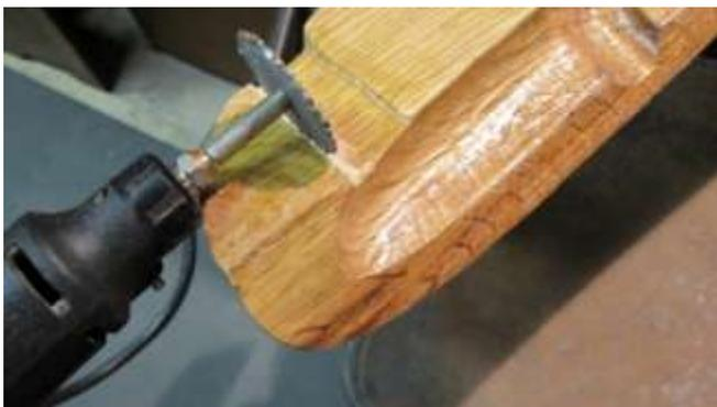
983. Sand the bow with 220 grit sandpaper then make a test fit again and mark the locations that need trimming. Trim with a saw blade on a portable hand grinder after a final fit.
