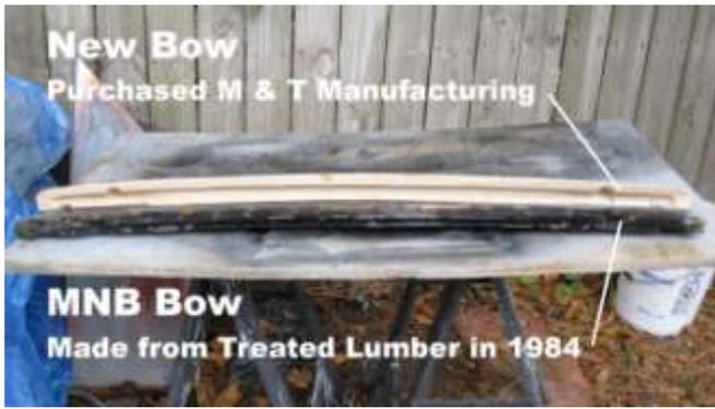
980. A view of the new wood bow as purchased from M & T Manufacturing and the bow I made in 1984 from treated lumber. Mine worked fairly well, but I decided to go with a new one this time. The new one is slightly smaller.
