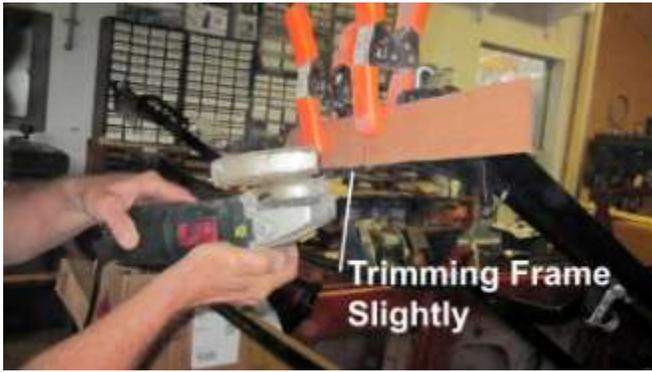
992. Vic, trimming the top of the frame, slightly, with an angle grinder.
