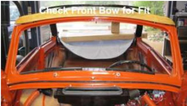
993. A final check of the bow for fit, again, prior to installation.
