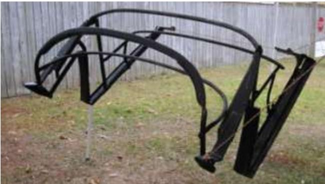
966. Wipe the frame down with wax and grease remover and hang the frame to make it easier to paint.
