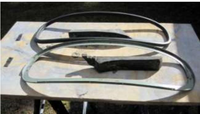
967. Prepare the rear window metal frame and new wood insert for painting.
