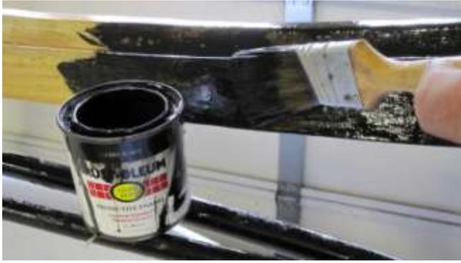
996. Carefully paint the wood bow and front frame bracket, especially where the sliver was cut off with Rust-Oleum gloss black enamel paint.
