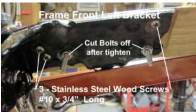
995. From the back side attache 3 additional stainless steel wood screws #10 x 3/4" long. After all is tight and you are satisfied with connection & fit, cut off the excess bolts length as shown.
