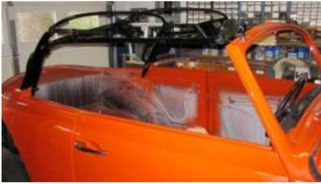
984. Place the frame on the body and make sure it is sitting square in order to correctly set the bow.
