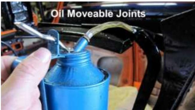
989. Oil all of the moving joints or connections on the frame.
