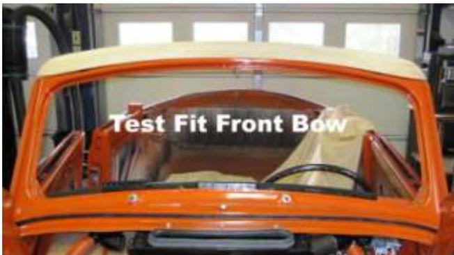
978. Test fit the bow on the window frame.
