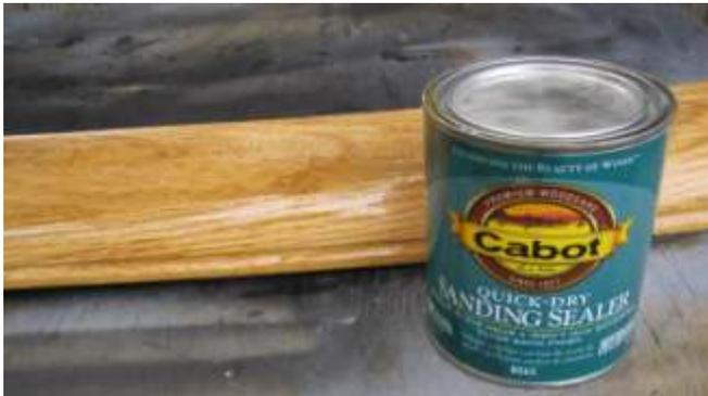
982. Paint two coats of sanding sealer waiting overnight for the second coat. Sand each coat lightly with 120 grit sandpaper.
