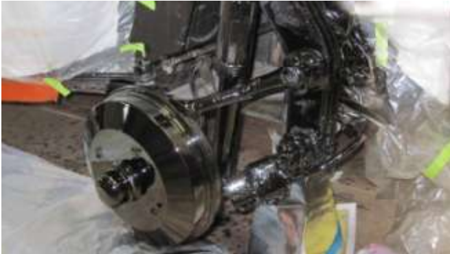
950. A view of the front wheel hub completed.
