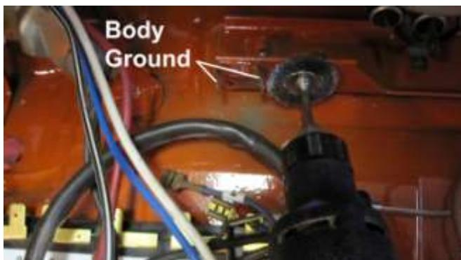
895. Clean the paint off the body ground connectors with a wire brush on a hand grinder.
