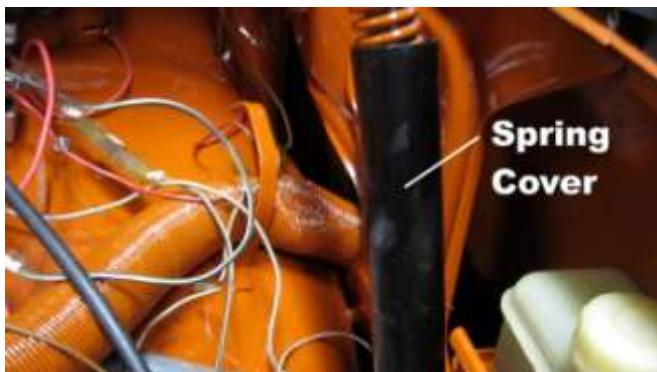
929. Install the spring cover over the hood support springs.
