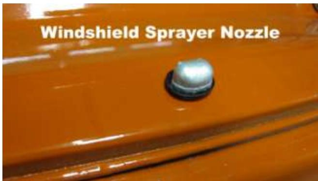
932. Install the sprayer nozzle and connect the hose from the wiper switch.
