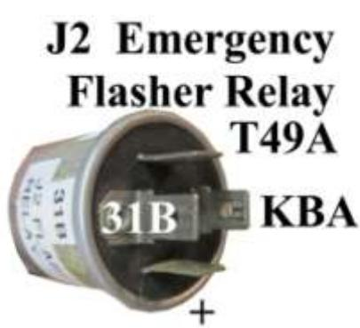
883. A detailed diagram of the emergency flasher relay, with wire connections shown.
