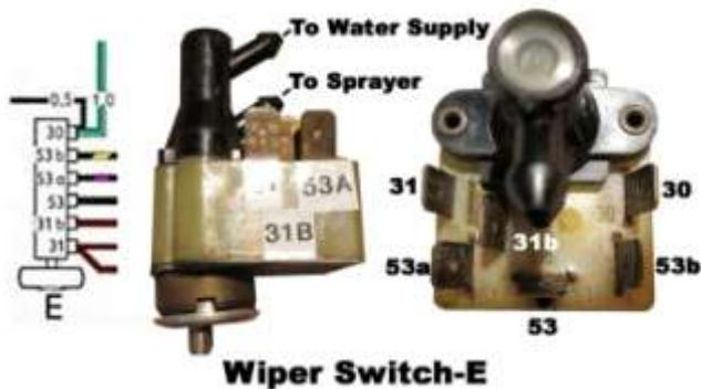
888. A detailed diagram of the wiper switch with, wire connections shown.
