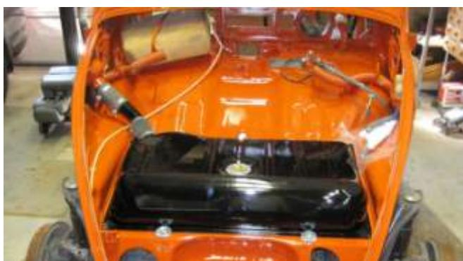
867. The gas tank now reinstalled.
