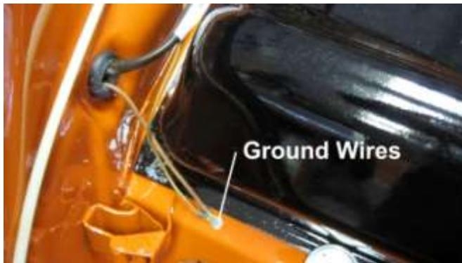
876. Connect the ground wires for the parking lights and the headlights on the right side of the trunk.
