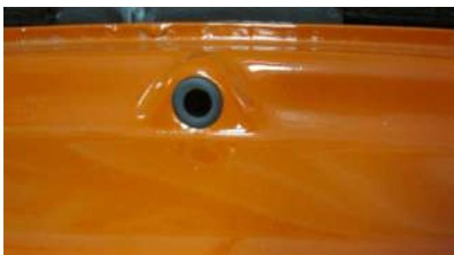
919. Install new rubber grommets in wiper arm holes.
