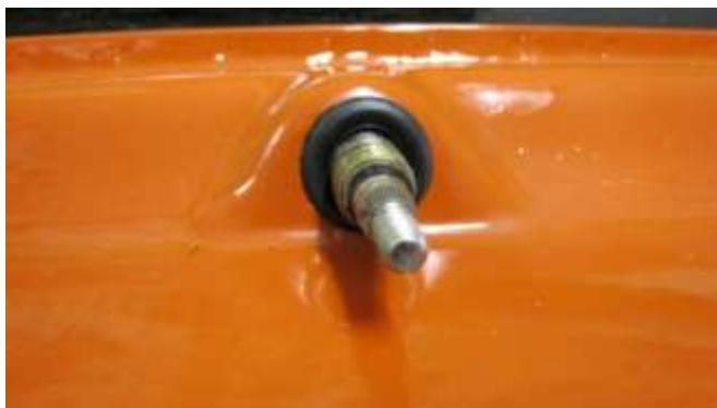
920. Install the wiper assembly by pushing up in the trunk and out the wiper arm holes.
