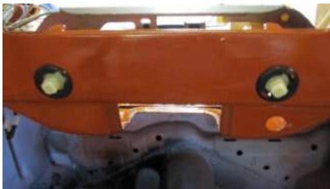
872. Install the retainer rings for the fresh air control knobs.
