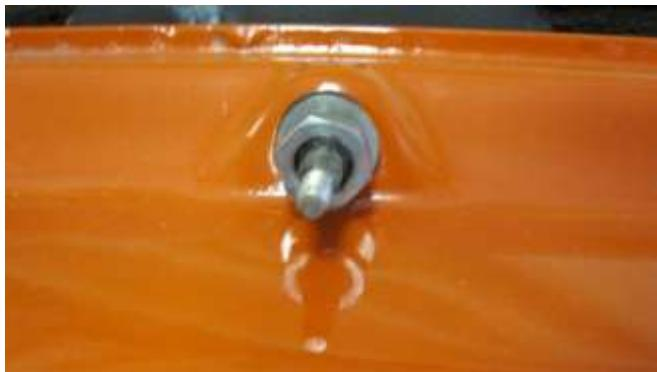
921. Insert the washer and nut on each wiper arm.
