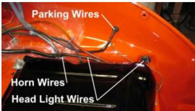
877. Install the parking light wires and the headlight wires on the left side of the trunk by pushing the wires in from the fender well side.
