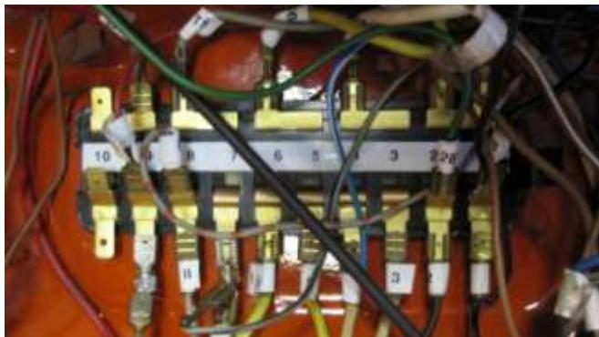
909. Final fuse block shown as installed. Check & double check the wires vs. the wiring diagram shown on page 21. Add gas to the gas tank, install the battery, and crank the Engine. Yes, it CRANKED and no SPARKS!
