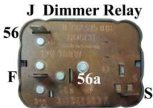
914. Detail of the dimmer relay, with wire location shown.
