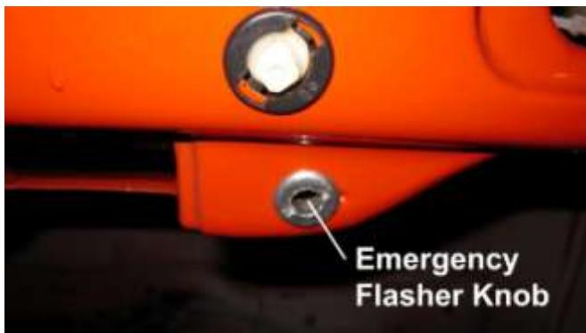
880. Install the emergency flasher switch and wires, shown from inside the car.
