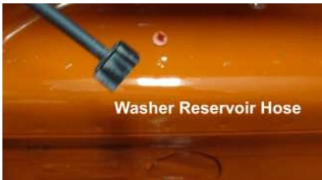
926. Route the supply line to the windshield washer tank location as shown.
