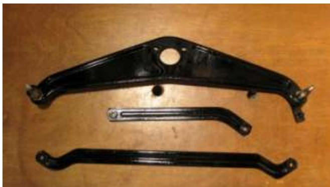
916. Clean the wiper assembly and paint any paintable parts.
