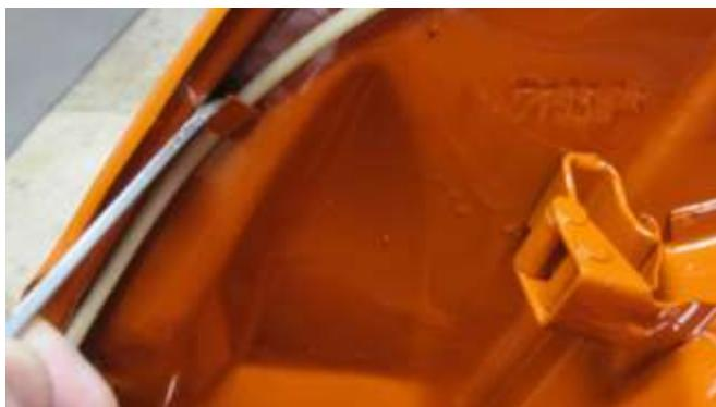
868. Bend closed the cable clip for the hood release cable with a flathead screwdriver.
