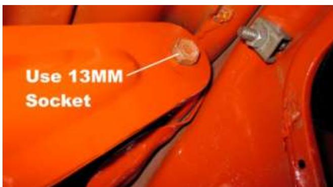
927. Use a 13 MM socket and install the hood support arms top bolt.
