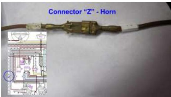
908. Install Connector "Z" - Horn
