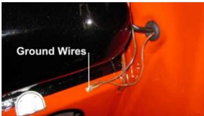
878. Connect the ground wires for the parking lights and the headlights on the left side of the trunk.
