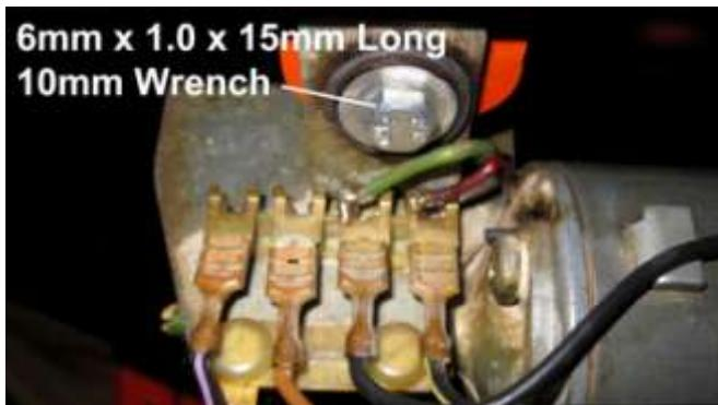
923. With a 10mm wrench connect the wiper motor to the car body then connect the electrical wires between the wiper motor and wiper switch, as shown below.
