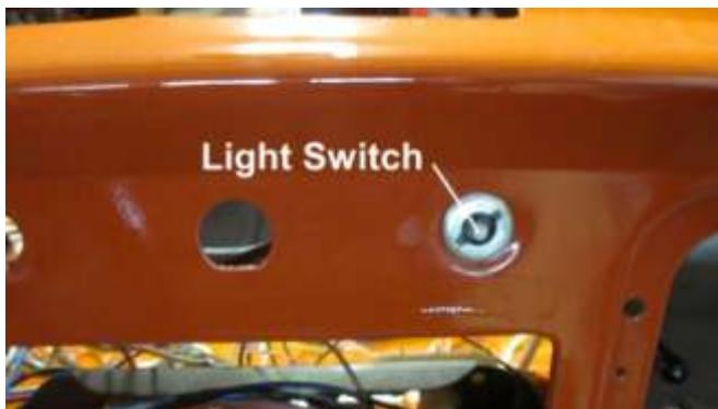
884. Install the light switch and wires, as shown from inside the car.
