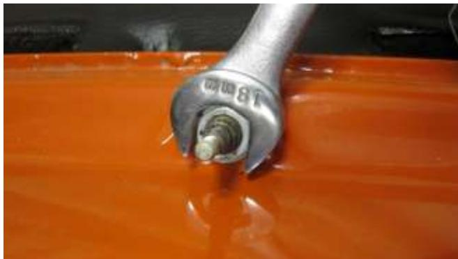
922. Carefully, tighten the wiper nut with a 18mm wrench, but don't mess up that paint job.
