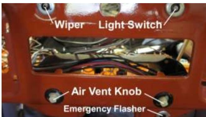
887. Install the wiper switch and wires.
