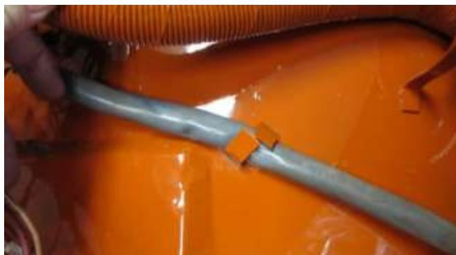
890. Carefully, close the main wiring harness clip in the trunk.
