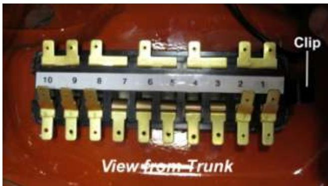
894. As shown for the trunk, install the fuse block with the fuse block clip.
