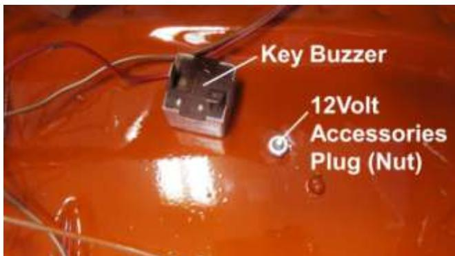
897. Install the ignition key buzzer in the trunk, as shown.
