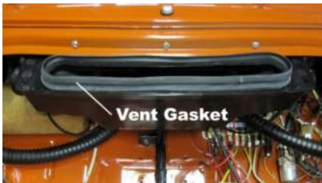
936. Install a new vent gasket on the fresh air vent box.
