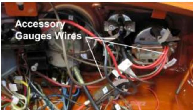
912. Install the accessory gauge wires.
