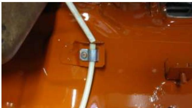
870. Fasten the cable clamp for the hood release cable from the pocket to the hood release catch. Place the pocket support block in place and position the pocket.
