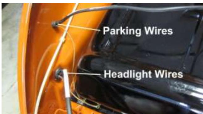
875. Install the parking light wires and the headlight wires on the right side of the trunk by pushing the wires in from the fender well side.
