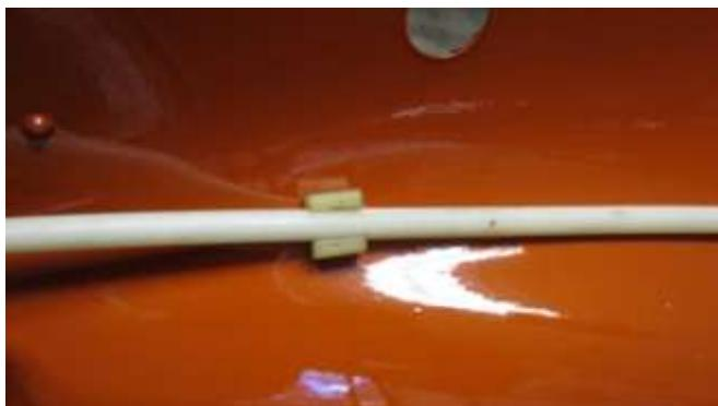
869. Carefully, snap in the cable clip for the hood release cable.
