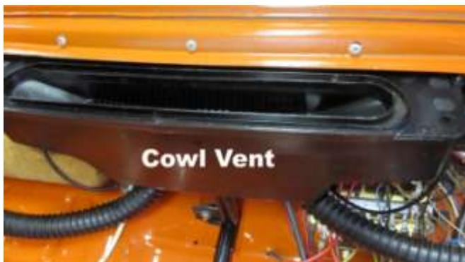
933. Install the cowl fresh air vent and connect the hoses, as shown.
