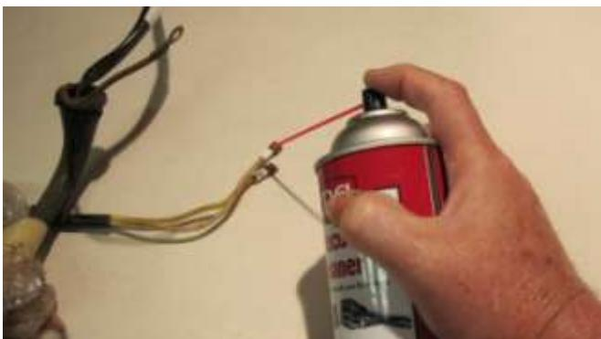
861. Start by cleaning each wire terminal with an electrical cleaner purchased at a local auto parts store. Also wipe down the length of the wire with WD-40 or silicon spray and then dry the wire.
