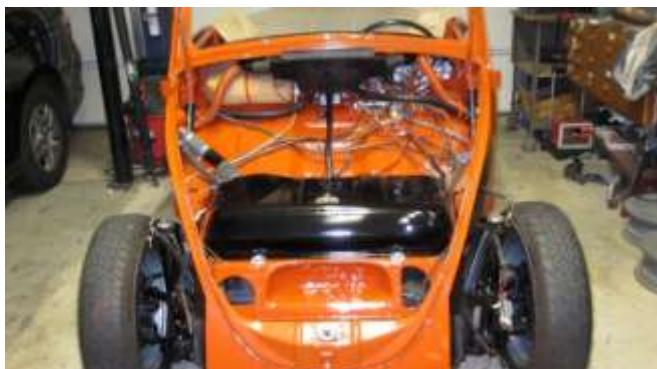
938. The electrical re-installation is now complete. All that is needed is to install the radio, speakers and the trunk lid.
