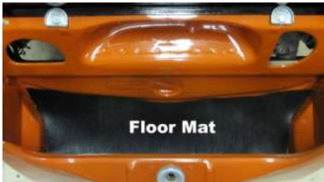
937. Cut out a floor mat to size to protect the spare tire area.
