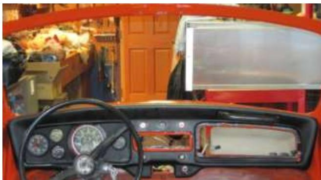
910. Install the dash then install the brake dash light.
