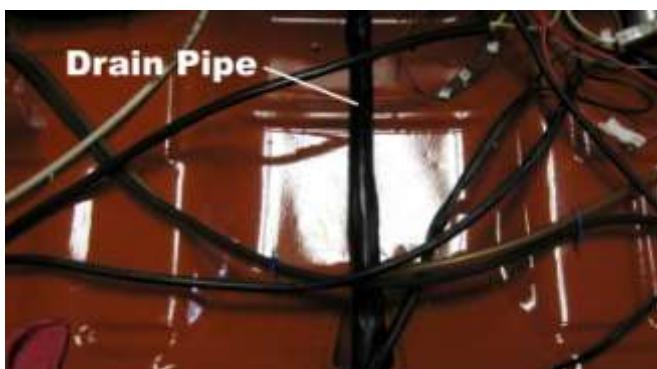
935. Extend the drain to the opening above the gas tank.
