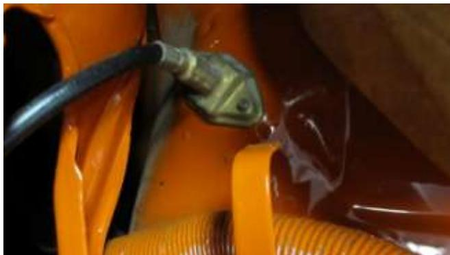
873. Install the cable unit for the gas tank door opener.
