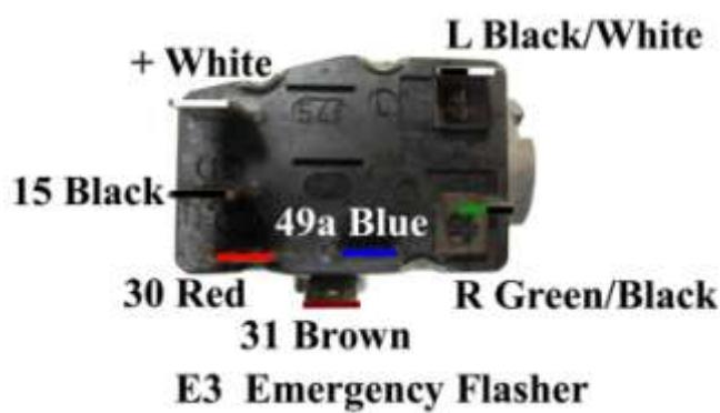
882. A detailed diagram of the emergency flasher switch, with wire connections shown.
