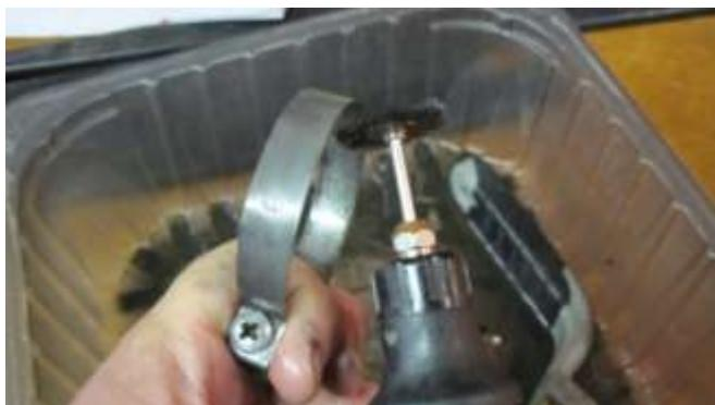
865. Clean the gas tank filler tube clamps with WD-40 and polish with a steel wire tool on a hand grinder.
