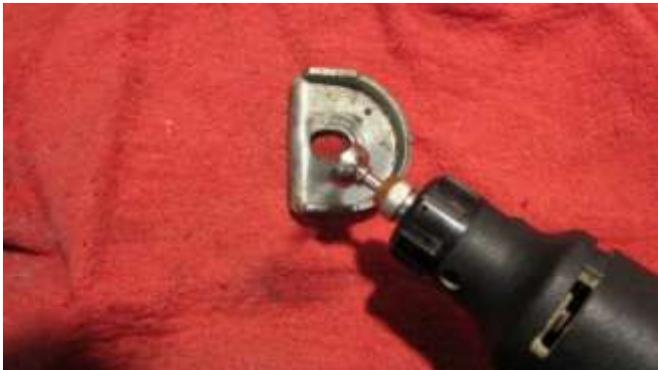
863. Clean the gas tank hold down connectors with WD-40 and polish with a steel wire tool on a small hand grinder prior to installing on the car..
