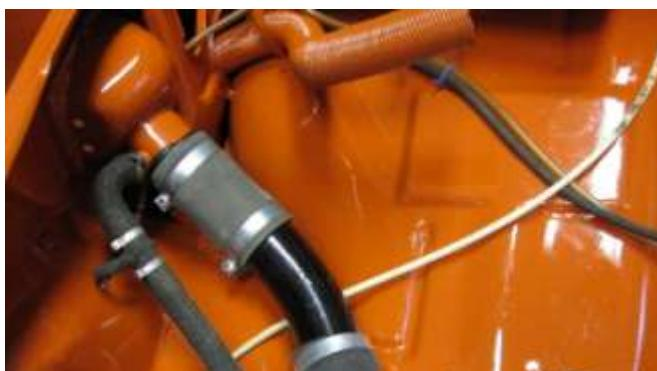
866. Install the gas tank filler tube and overflow tube.
