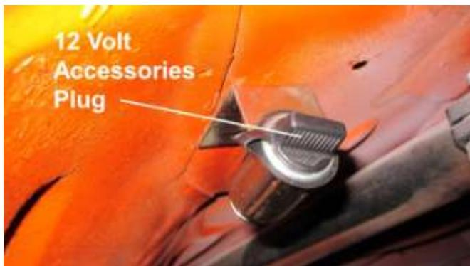
896. Install the 12 volt accessory plug under the dash.
