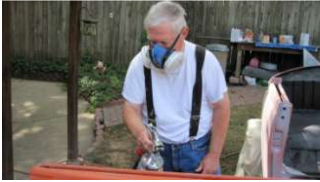
620. Malcolm painting inside of the door of the car with a tack coat of prime.
