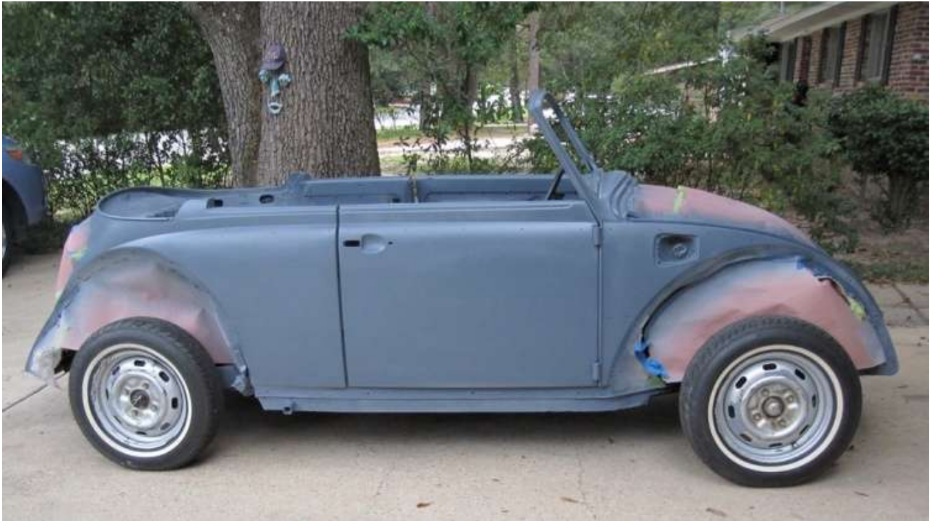
632. The exterior, after painting the prime seal coat.
