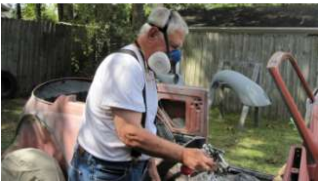
619. Malcolm painting the inside of the car with a tack coat of prime.
