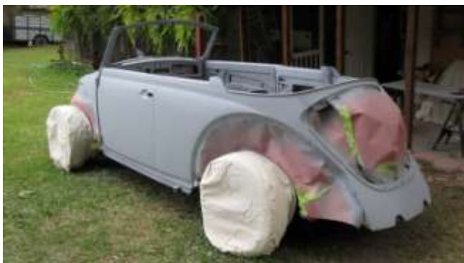
623. Rear of the car with a second coat of prime painted.
