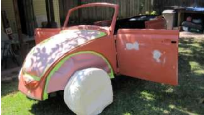
617. Front of the car masked up, as shown. The tires were covered with tire covers.
