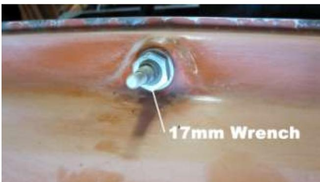
581. With a 17mm wrench remove the large nut and washers on each windshield wiper arm.
