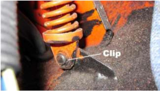
578. Remove the clip on the bottom of each hood lever arm and remove.
