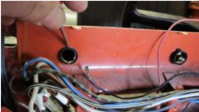
592. From the trunk, with a flat head screwdriver depress the ears on the fresh air assembly rings to push the rings inside of the car to remove.
