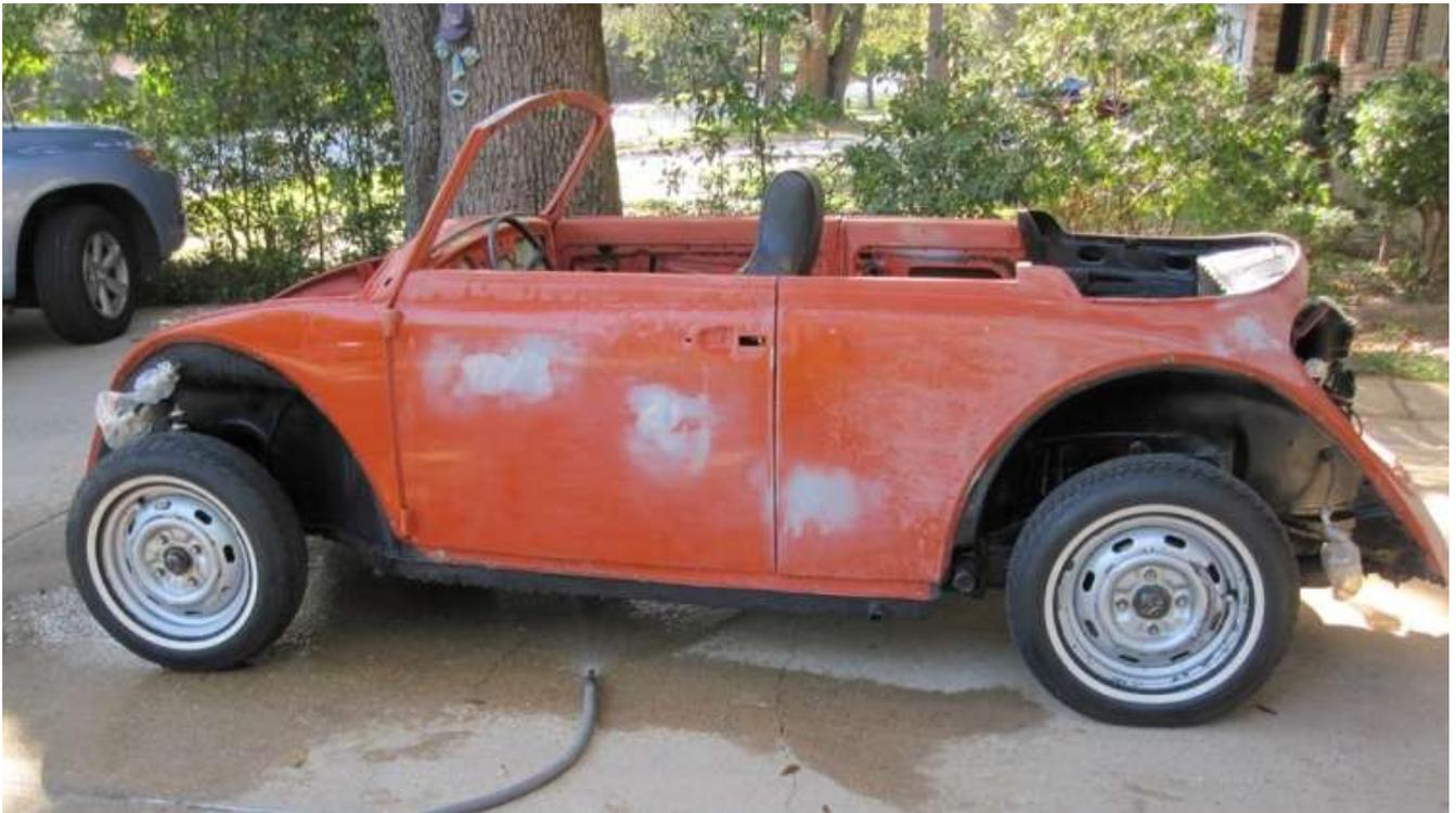
611. The body is now ready for masking and taping up for painting several coats of prime. See step 632 for body after painting prime and see step 764 for body after painting finish coat.
