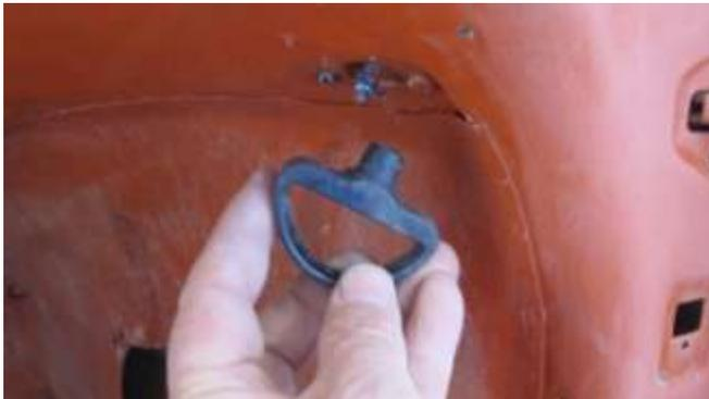
600. Unscrew and remove the gas tank door pull.
