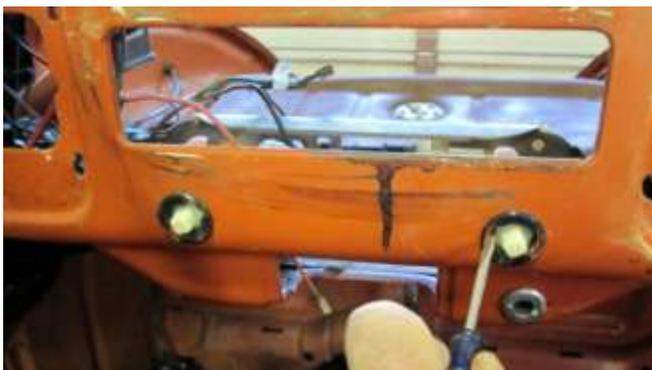
589. With a flat head screwdriver turn the fresh air knob rings to loosen the fresh air adjustment assembly.
