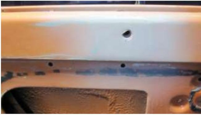
598. Apply filler to the seat belt scratches and then spray on prime to help find imperfections remaining on the scratches from the seat belt.
