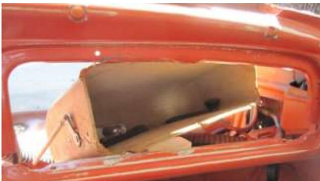
601. With an 8MM socket remove the pocket strap and push the pocked into the trunk.
