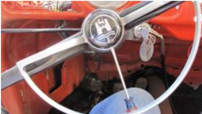
604. With a flat-headed screwdriver, carefully lift up the horn ring.
