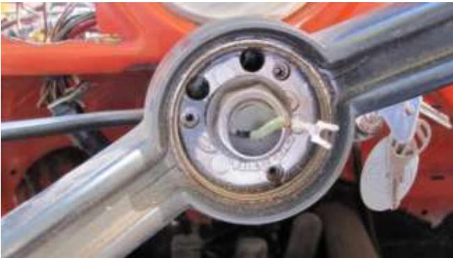
607. The disconnected green horn wire will remain as shown.
