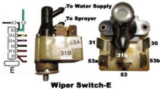
585. Mark both the wires and the wiper switch "E".
