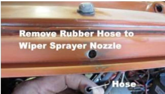
579. Remove the rubber hose connected to the wiper sprayer nozzle.
