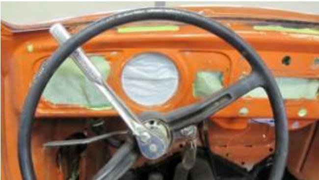
608. With a 1-1/16" socket, loosen the steering wheel nut but don't remove.
