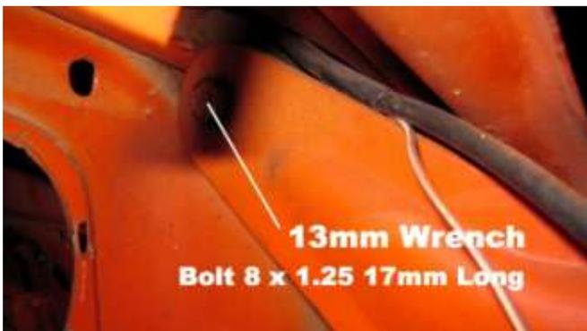
577. Remove the remaining items from the body such as the hood lever arm by removing the top bolt on each hood lever arm and with someone holding the hood then remove the remaining two bolts.
