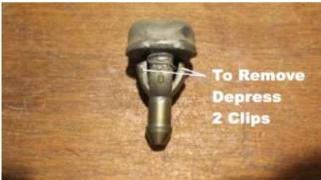
580. From within the trunk with a screwdriver depress the clip sides on the sprayer nozzle and push the nozzle up out of the car.
