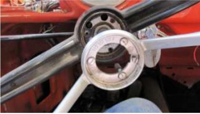
606. Lift the horn ring off the steering wheel, clean up, tag bag, and store the horn ring parts.
