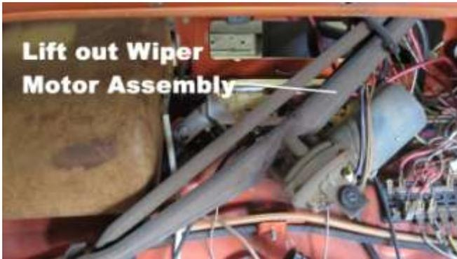
583. Lift out the wiper motor assembly.
