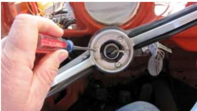
605. With a flat-head screwdriver remove the three screws holding the horn ring. The horn wire will be connected to one of the screws, and disconnected as you remove the screw.
