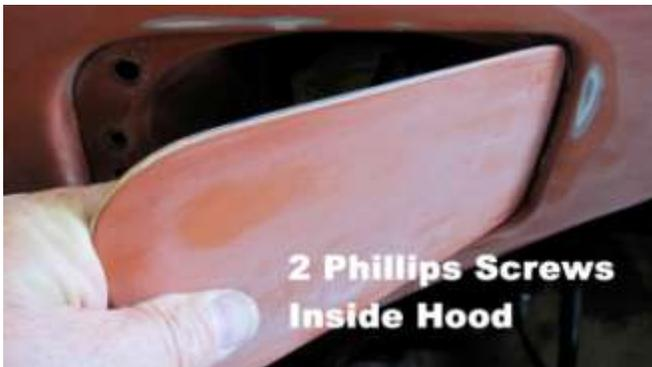
588. From within the trunk, remove the two Phillips screws holding the gas filler door.
