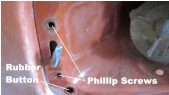
587. With a Phillips screwdriver, remove the screws to the gas filler door lock assembly, and push it into the trunk. With pliers, pull out the two rubber door bumpers.
