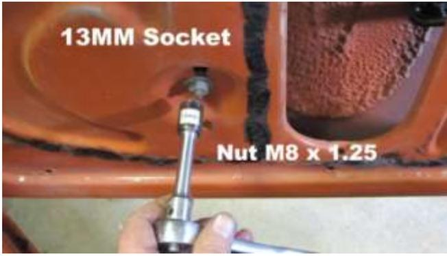
465. With a 13 mm socket remove the lower nut to the front window guide frame.
