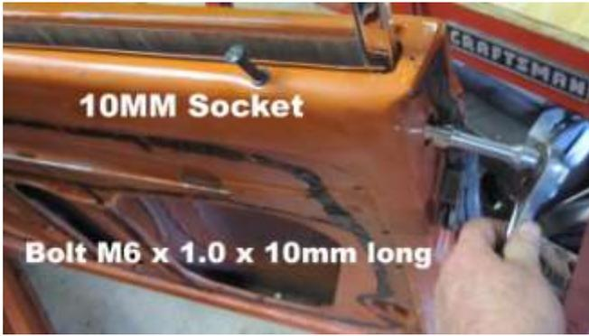
461. With a 10mm socket remove the upper bolt to the rear window guide frame.
