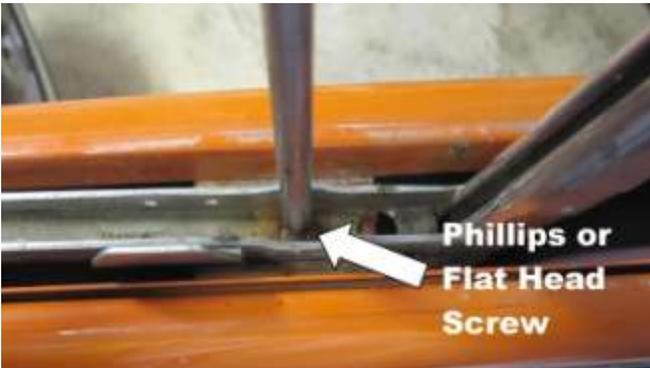
458. With a screwdriver remove the vent window hold-down screw.
