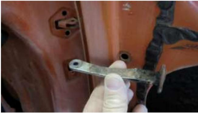
489. Remove the door pin and lift out the door latch connection form inside the door. Right side shown. Also remove the latch for the left side
