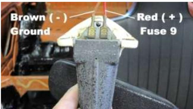
484. The rear view mirror was removed and electrical wires labeled as shown.
