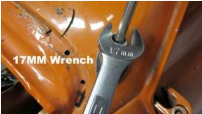
482. With a 17MM wrench, remove the nut on the radio aerial.
