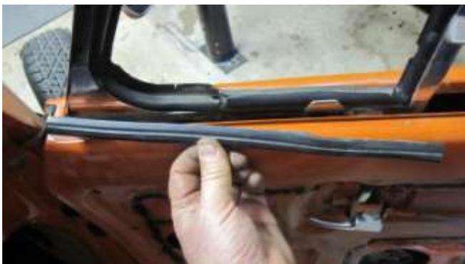
456. Remove the inside vent window rubber.
