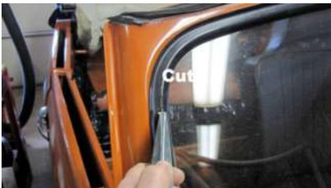
476. With a razor blade knife, cut the rubber molding as shown above, around the entire perimeter of the windshield.
