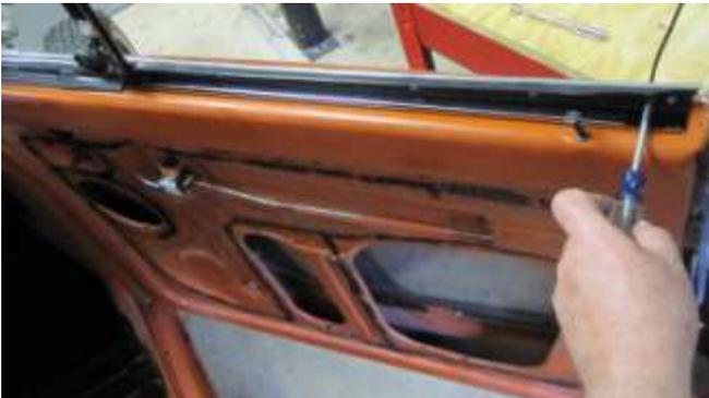
459. Lower the front window and remove both inside and outside window scrapers.
