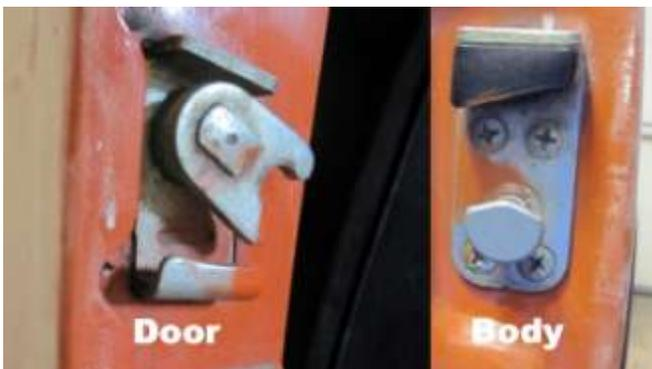
487. With a large Philips screwdriver remove the M6 x 1.0 x 15mm long screw on the latch on the door and push inside the door to remove. Remove the latch on the body, and clean up and label both and store.
