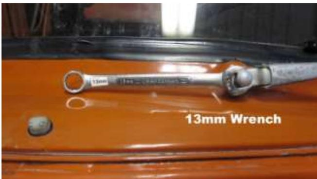
472. With a 13MM wrench remove the windshield wiper nut.
