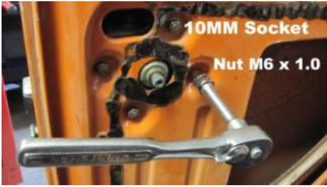
453. With a 10 mm socket remove the four nuts to the window crank.
