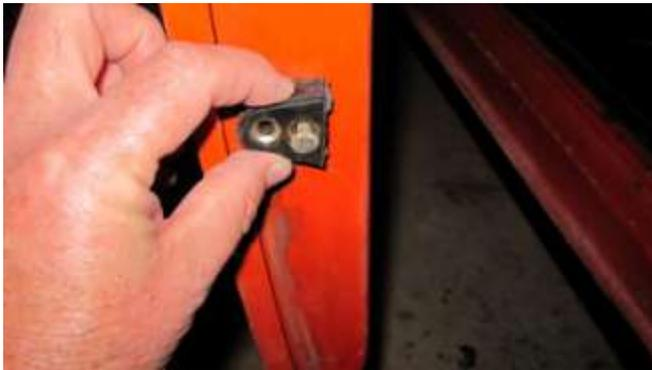
486. With a large Philips screwdriver remove the M6 x 1.0 x 15mm long screw on the door jam and remove the door alignment guide. I left the door handle and striker plate on at this time since I will be driving the car around to the back yard. If your car will remain stationary, go ahead and remove the door handle and striker plate as shown below.
