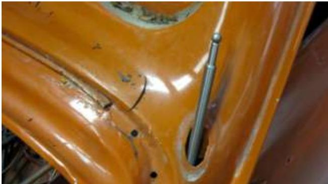
483. Push the radio aerial inside the trunk to remove.
