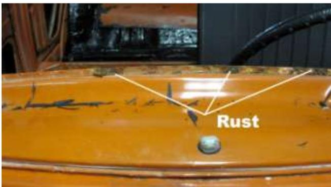
480. There was evidence of a small amount of rust, so taking off the windshield prior to finishing was a good idea.
