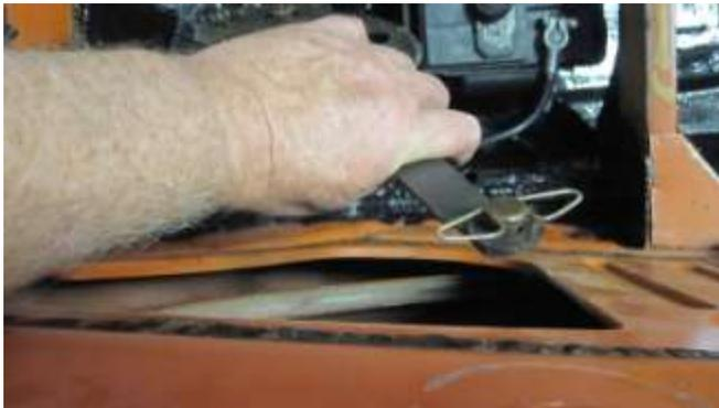
454. Remove the window crank mechanism. Clean up all right rear window pieces and tag and bag all parts remove and label as right rear window.
