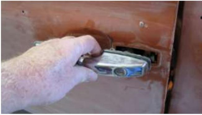
485. With a large Philips screwdriver remove the M6 x 1.0 x 10mm long screw on the door jam and slide the handle horizontal to remove the door handle.
