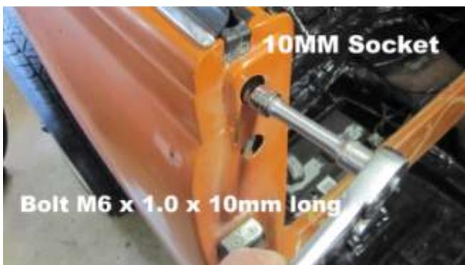
451. With a 10mm socket remove the two window bolts.
