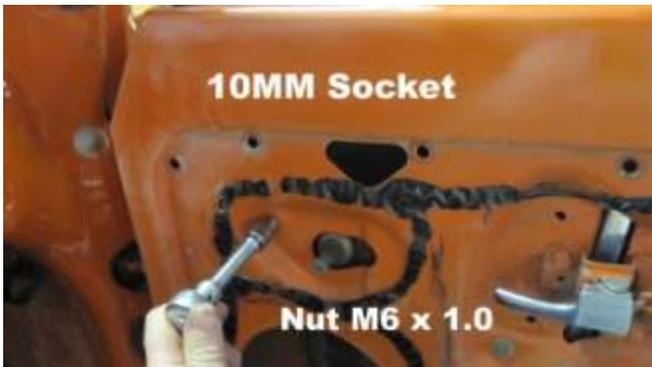
463. Remove the three nuts to the window crank mechanism so it can be moved out of the way of the window frame.
