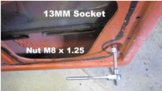
462. With a 13mm socket remove the lower nut to the rear window guide frame. Then lift the guide frame out of the car.
