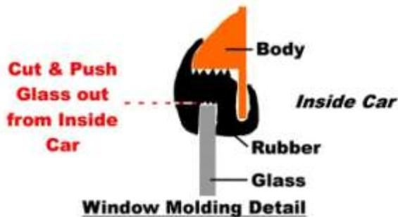
475. I chose to cut the rubber molding as shown and then lift the window out.
