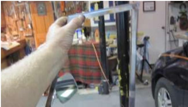
466. Then lift the window guide frame out of the car. You will also need to twist as shown below.
