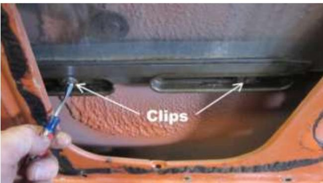
460. Remove the two window clips and pull the window up and out of the car.
