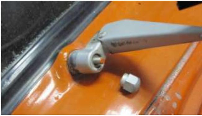
473. With the nut removed, lift off the entire windshield wiper.
