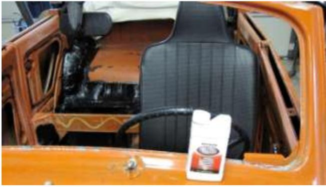
481. Sand as much of the rust off as possible and then paint rusted areas with Rust-Oleum rust reformer.
