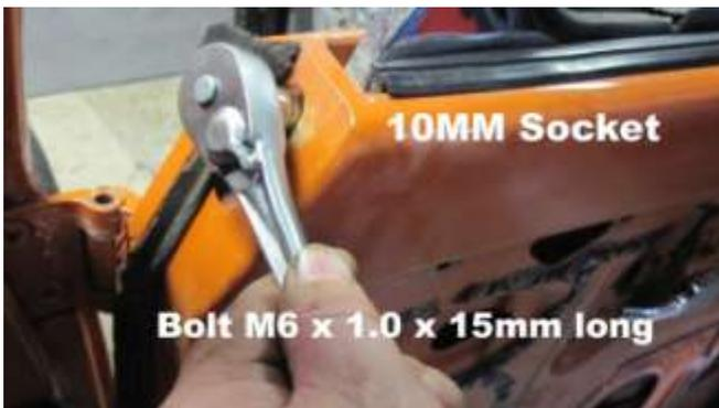
464. With a 10mm socket remove the two upper bolts to the front window guide frame.
