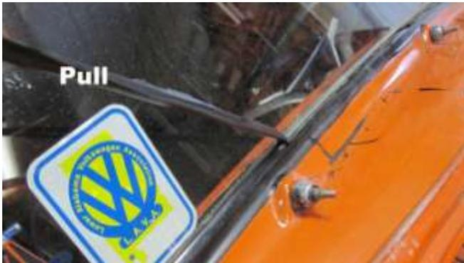
478. Pull off the cut strip around the entire perimeter of the windshield.
