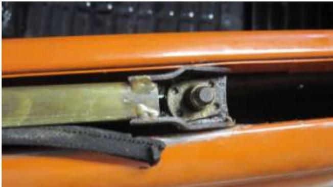
467. Twist the window guide frame as shown so it can be pulled through the window opening. Note when reinstalling this frame you will have a new paint job so be very careful and do not scratch the new paint job. Remove the window crank mechanism.
