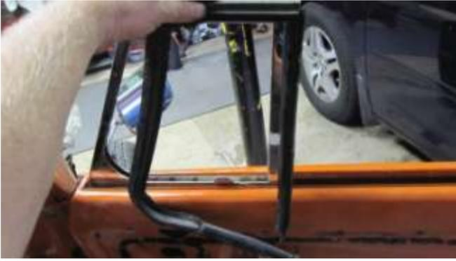
457. Remove the vent window rubber as shown
