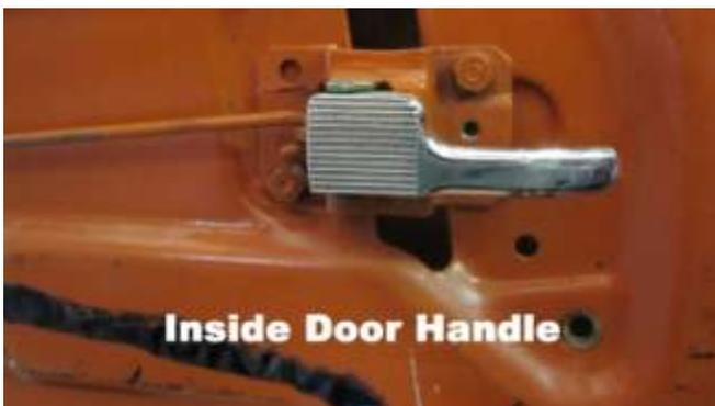
488. Remove the inside door handle and mechanism.
