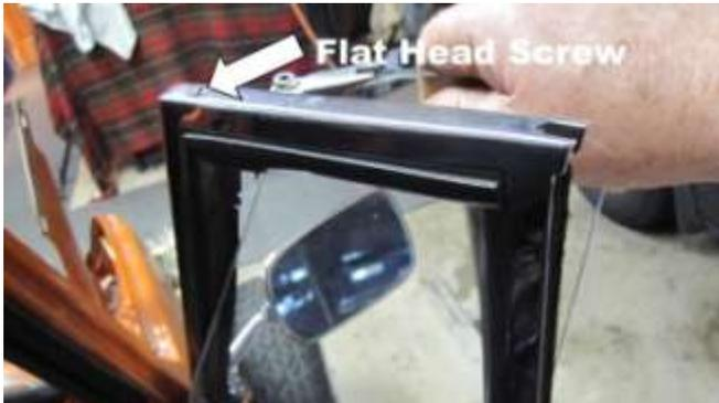
455. With a flat-head screwdriver, loosen the top screw enough that the vent window will pop out of the frame and then lift the window out of the frame.
