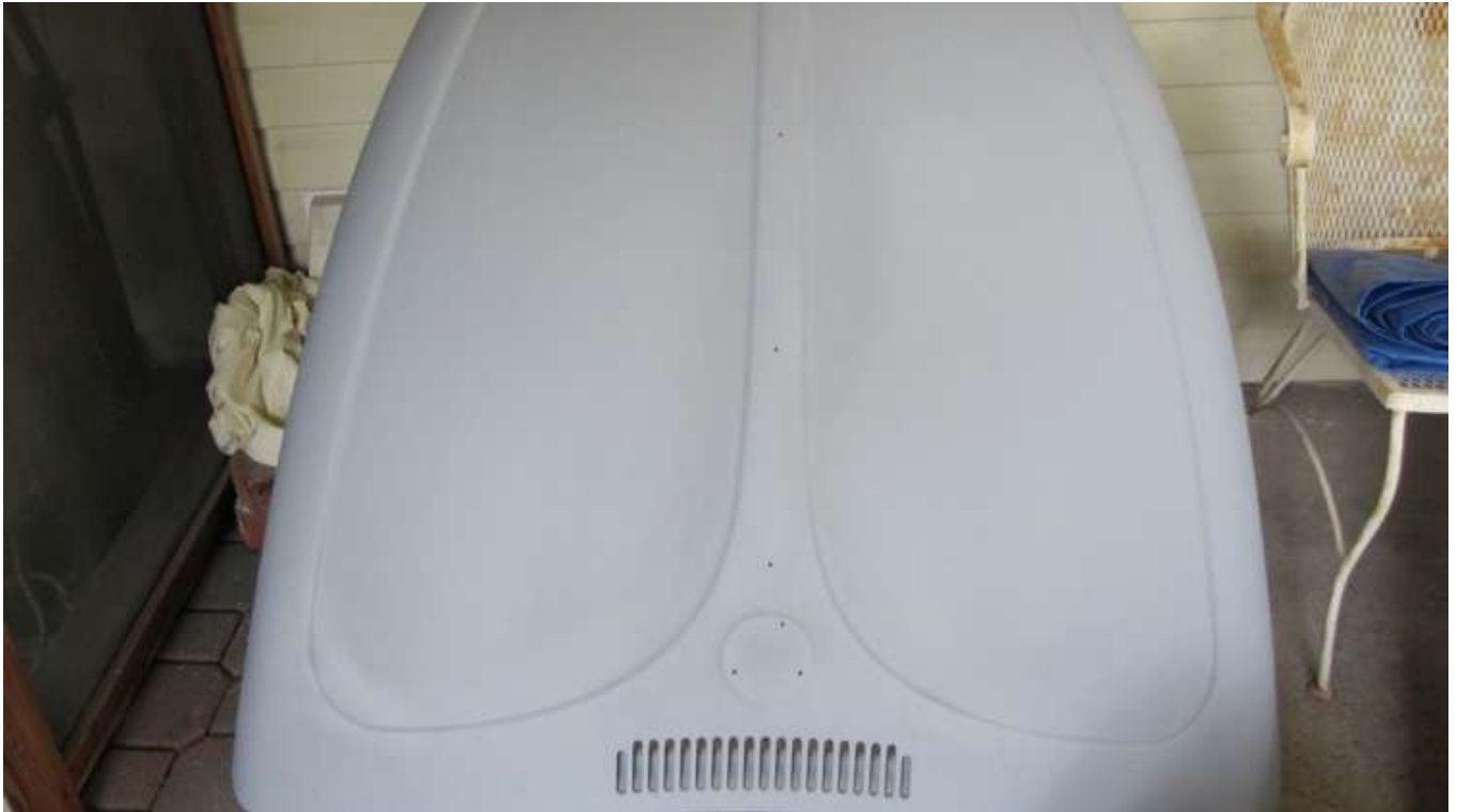
448. Front side of hood after four coats of prime.
