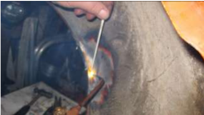
341. Walt, welding the crack on fender.
