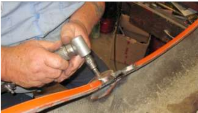
342. Walt shaping the weld area.
