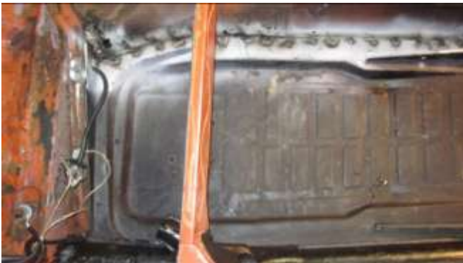
230. Passenger side rear: welds completed.
