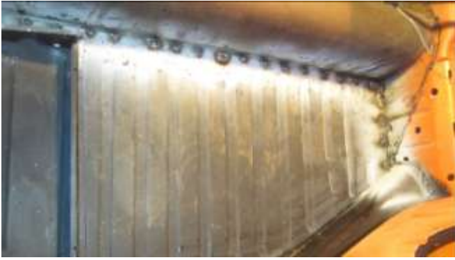
229. Passenger side front: welds completed.
