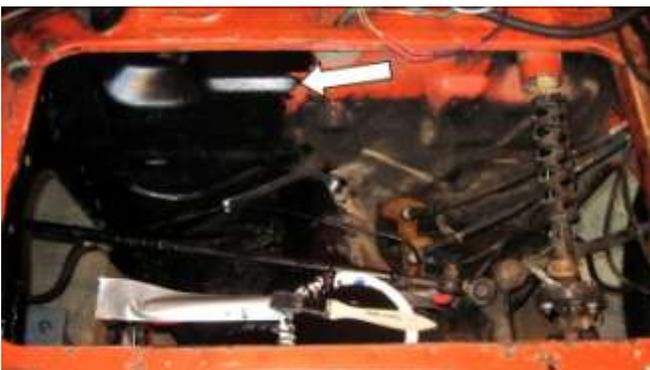
197. After the area has dried completely, usually overnight, begin painting the firewall with the Eastwood rust encapsulator paint, as shown below.
