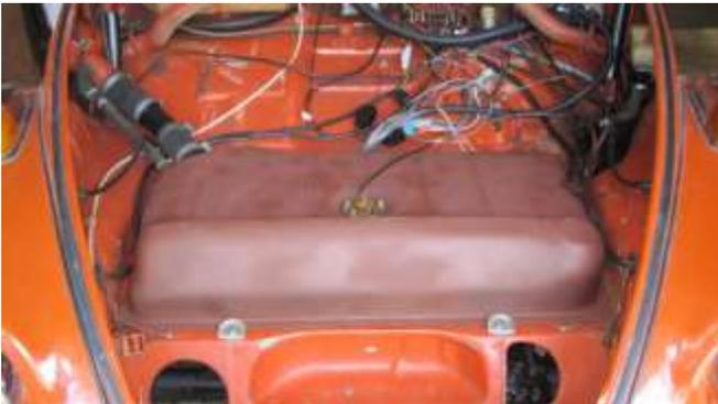
212. The fuel tank is finally reinstalled as shown.
