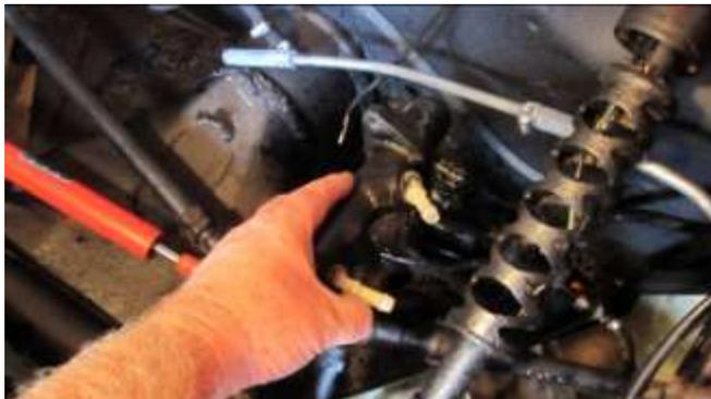
204. From the front of the firewall side, remove the brake master cylinder.
