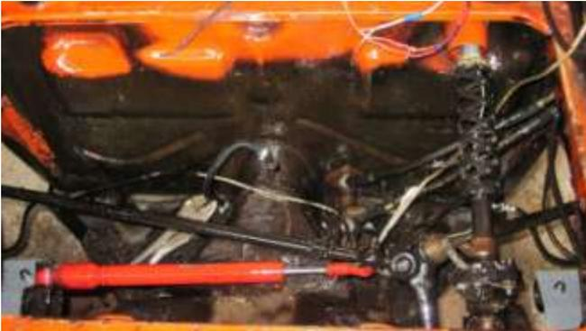
195. After 10 - 15 minutes wash the area down with a water hose, which is easier if the car is outside in the open. Note: be careful not to get water on the dash electrical area.
