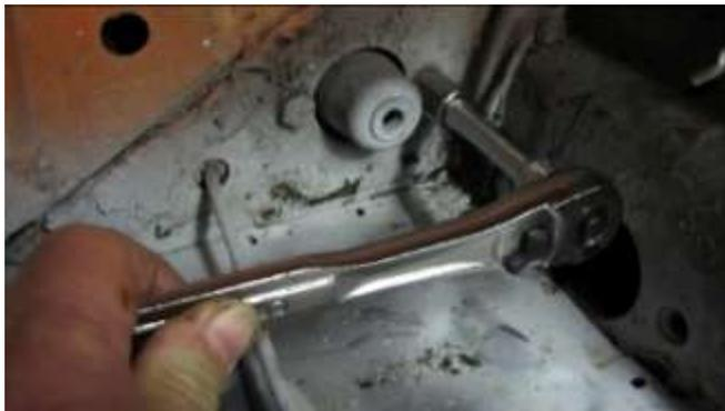
203. I decided to go ahead and replace the brake master cylinder while I was here. I disconnected the brake lines to the master cylinder and the stop light wires and then removed the two 13mm bolts from inside the car to disconnect the master cylinder.
