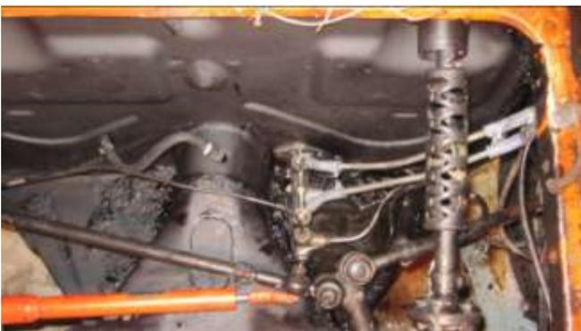
209. The brake lines were installed and then the stop light switches connected and the brake fluid line connected.
