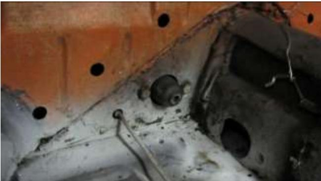
208. Two bolts for this assembly were installed with a 13mm socket from inside the car.
