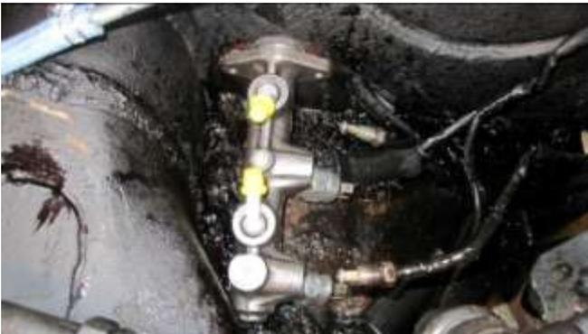
207. Then the new unit was set in place in the front firewall opening.
