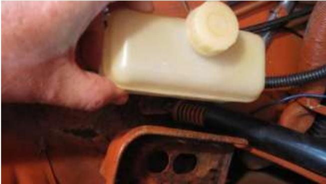
199. Remove the brake fluid reservoir and clean the bracket and hoses.
