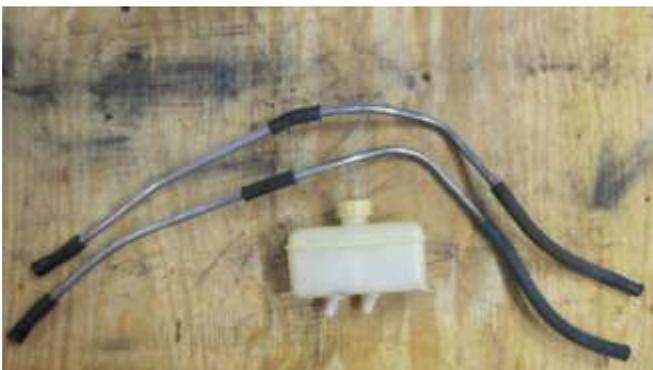
201. Remove and clean the brake lines and reservoir tank. It is best to install new rubber brake hoses at this point.
