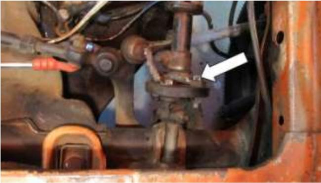
191. Using two 14MM wrenches, connect the two bolts to the steering column.
