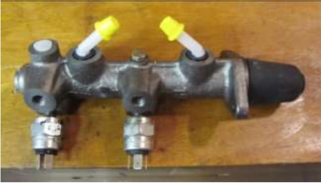
206. Install the brake stop light switches on the new unit as shown.
