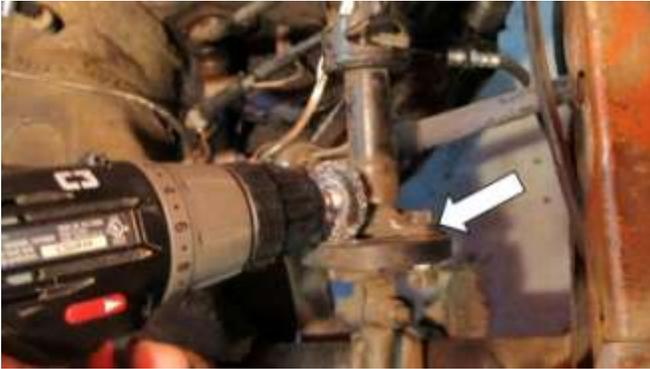
190. Prior to connecting the steering column clean the horn wire terminal and connection location with sandpaper or a wire brush, as shown.
