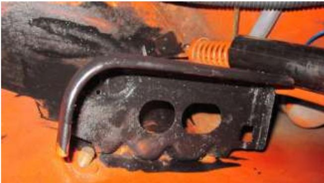
200. Remove as much rust as possible, with sandpaper and steel wool, then paint the brake fluid bracket with Eastwood rust encapsulator paint.
