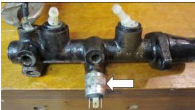
205. Remove two stop light switches from the old master cylinder to install on the new master cylinder. Note: picture shows one already removed.
