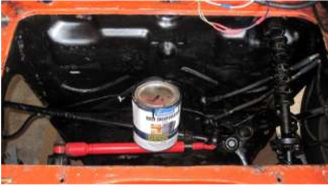
198. Firewall and metal parts painted with Eastwood rust encapsulator paint.
