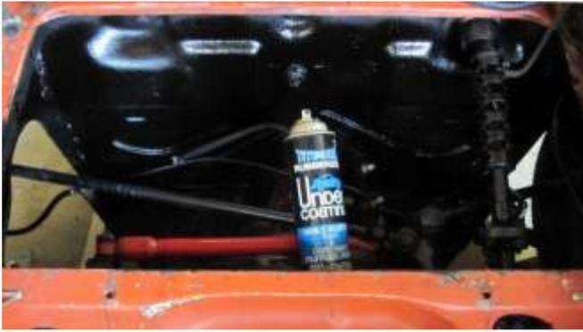
202. I sprayed the firewall with a rubberized undercoating. Rust will win in the long run, but this may delay it.
