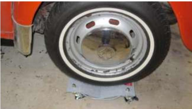
193. I used dollies on all 4 wheels to turn the car around, and move the car to desired location, this required jacking the car up to allow dollies to be slid under each tire.
