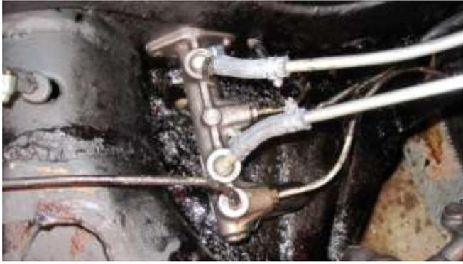
210. New brake line hoses with clamps, as shown.
