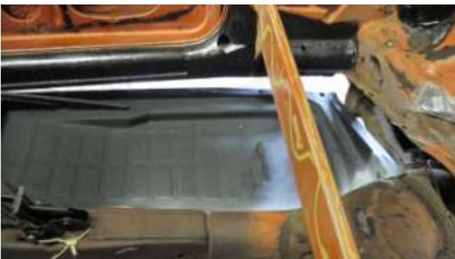
171. The passenger pan slid into place over the rack on the frame in the rear.
