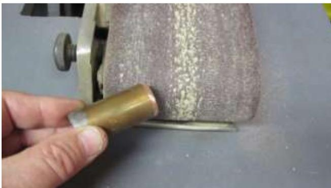
179. My seals came without bolts holes cut, and I did not have a punch large enough so I sharpened one end of a 1/2" diameter pipe sleeve to make a punch. I am not strong enough to push the point of the floor pan bolts through the rubber.
