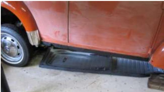
166. I slid the passenger pan under the body for a trial fit.
