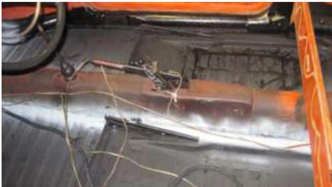
182. Finally, I was able to get the pan to lay generally flat so I could start installing the body bolts.
