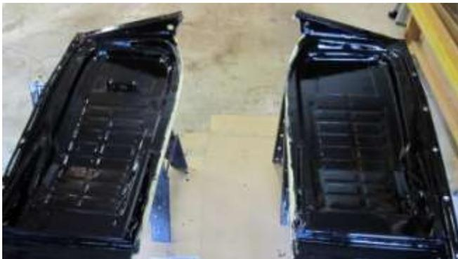
145. The second coat of POR15 completed for both pans. A Third coat of POR15 will be painted after the pans are fully installed.
