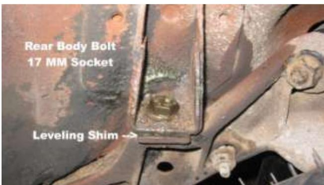
183. I started with the rear body bolts behind the rear fenders using a 17MM socket.
