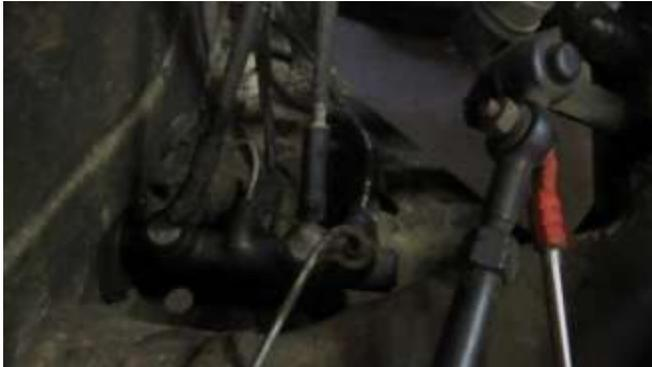
161. I did not disconnect the brake lines at this time since they were slip on type, but I will keep checking on this as I raise the car.
