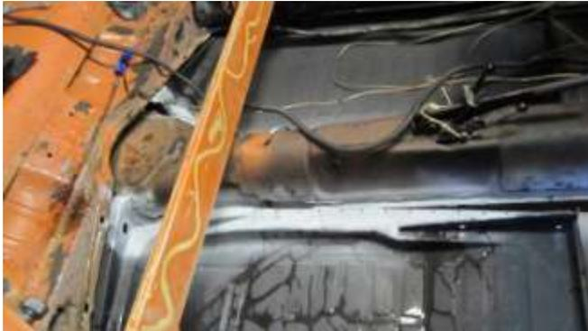
177. Both pans are now in place for a test fit, but not connected. The body was lowered back down on the chassis, but not all the way. The brake line was pushed through the pan hole and reconnected. No bolts installed yet.
