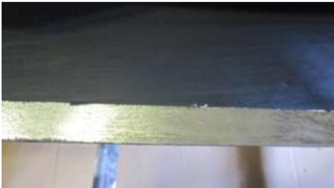
146. When the second coat has dried, remove the masking tape off of the future weld areas of the floor pans.
