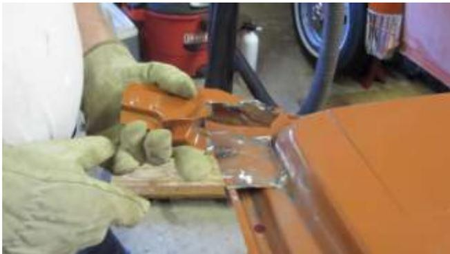
138. After a few cuts the jack stand was able to be lifted off, then the weld area could be cleaned.
