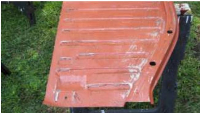
139. I wanted to remove the cheap factory prime. I did not want my POR15 put on a cheap factory paint that would come off, likewise my POR15 would also come off. I put on one coat of paint remover.
