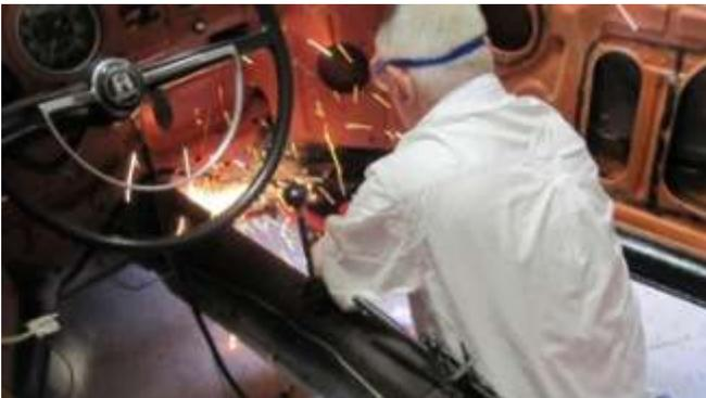
170. I cut most of the material out, but ended up cutting about 1/4 inch off of the right corner of the right pan and 1/2 inch off the left corner of the left pan, to make it work.
