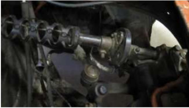
160. Disconnect the steering shaft and the horn wire using two 14MM wrenches.
