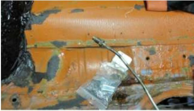
176. Pull brake line out of the way and place it as high as you can get it to minimize brake fluid leakage.
