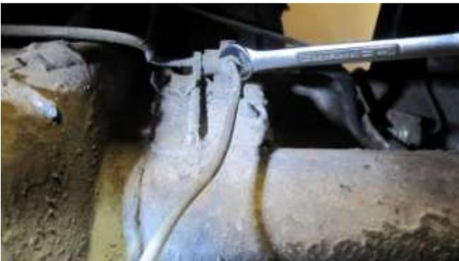
175. Disconnect the brake line to the rear of the driver side floor pan, with a 11mm wrench.
