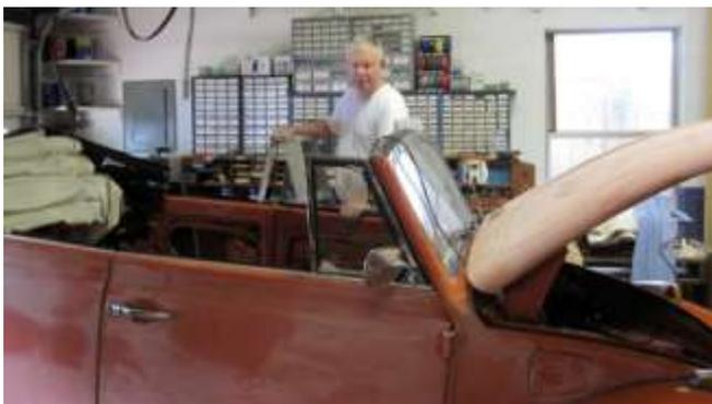
167. To keep from warping the body on a convertible shut and lock the doors. Use a ladder to climb in and out of the car. This would not be necessary on a sedan.
