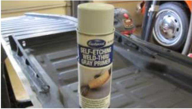
148. Use Self-Etching Weld-Thru Gray Primer and spray a coat over the future weld area.
