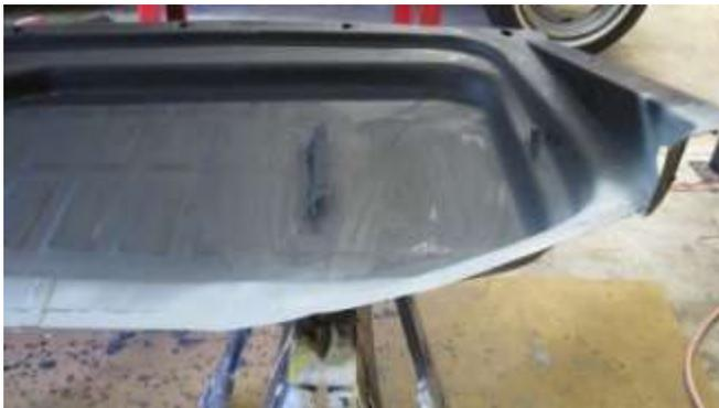
149. Pan shown with one coat of Self-Etching Weld-Thru Gray Primer sprayed over the future weld area.
