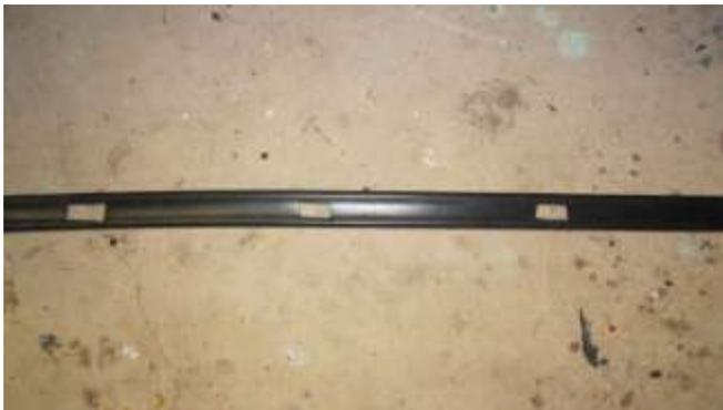
181. On the next side, I used a razor blade knife and cut the holes in the pan molding for the bolts, as shown.
