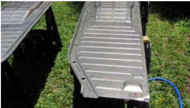
141. Three coats of paint remover, a little bit of elbow grease and the floor pan's are all cleaned up. Remember you should be ready to paint quickly since metal start to rust as soon as the air hits it with no protection on.
