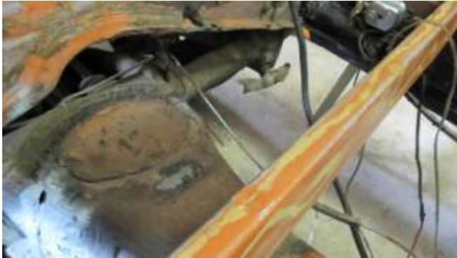
165. You can see the chassis is separated from the body about 4 to 5 inches. The front is only about 3/4".
