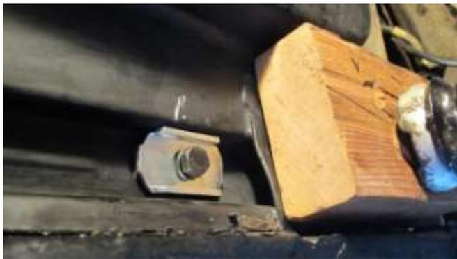
188. Finally, I was now ready to jack the pan tight to the frame and install the first pan bolt. A Total of 18 bolts.
