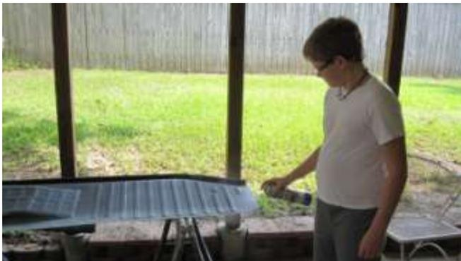
157. McNeil sprays on the self-etching weld-thru gray primer over the holes punched.
