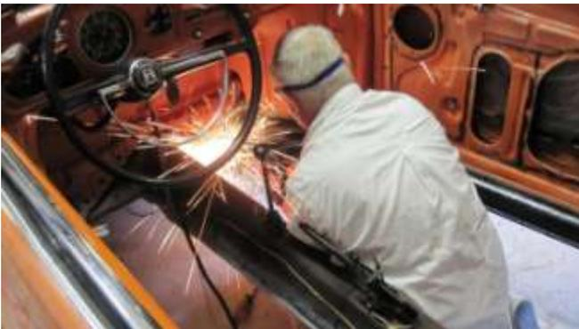
169. Before, I could install the pans there there was a little pan material in the front right corner that had to be removed.
