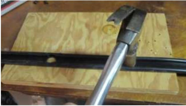
180. With sleeve and hammer I was able to cut the holes as shown. But, it is better to use a steel sleeve rather than the copper sleeve I used.
