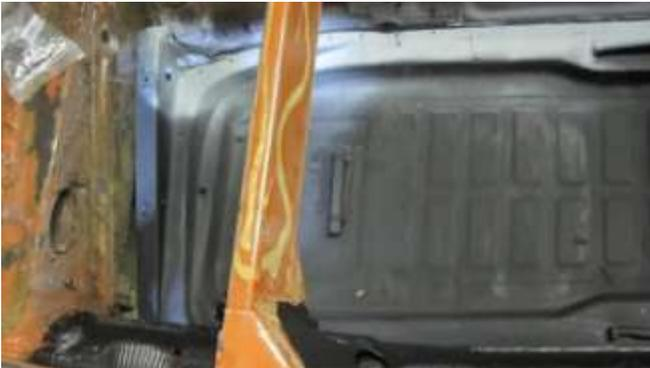
174. A view of the weld side on the rear portion prior to lowering the body in place. Now move to the driver side pan.
