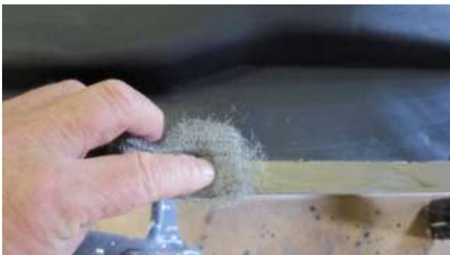
147. Rub the masking tape area down with steel wool to remove any tape residue.
