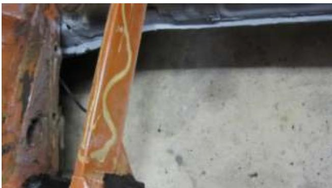
159. Before installing the pans, move back to the body and sprays on the self-etching weld-thru gray primer over the weld areas.
