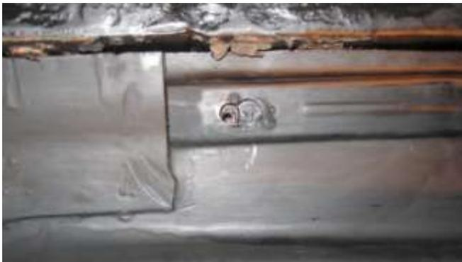
185. As you can see the factory hole did not match up with the body bolt hole so I had to drill/cut an adjacent hole. This was very time consuming with the pan on the body. I have gone back to step 137 and suggested that you make these holes oblong prior to installing the pans. Or you can install the pans, mark them, and remove them, to cut the holes and then re-install the pans.
