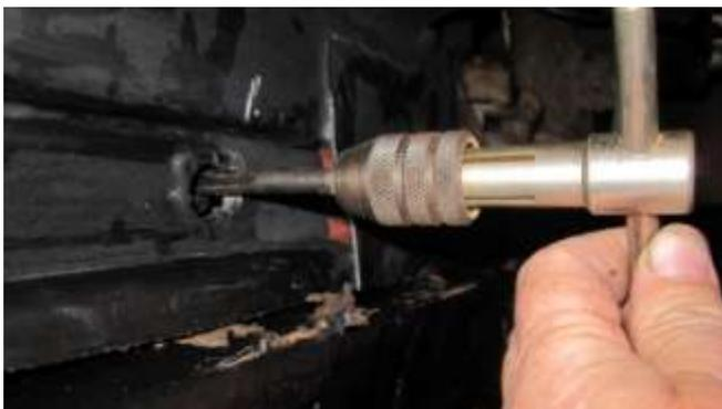
187. To make sure I did not have any paint or debris in the bolts holes I sprayed the hole with lubricating oil and ran a metric 8 x 1.25 tap in each holes to repair the threads. Note: One bolt, the third back from the front on the driver side, appeared to be oversized, apparently from the first restoration, so use a 15MM socket on this bolt, and if it is ever removed, put it back in the same position.
