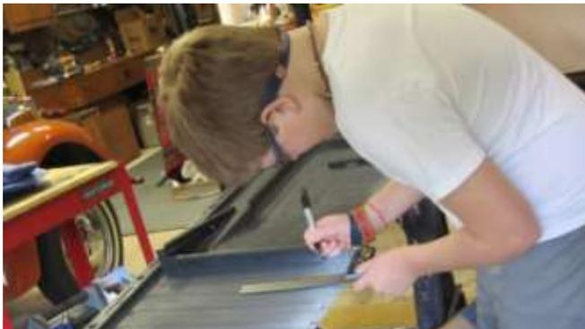
150. Grandson McNeil, marking layout lines for the punch holes.
