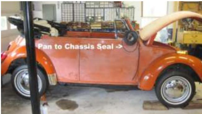
178. Raise the car again and put the car on jack-stands so you can install the chassis seal between the pan and the body.
