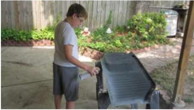
156. McNeil spraying on the self-etching weld-thru gray primer over the holes punched.
