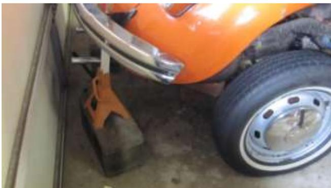
163. Then lower the car. The chassis dropped about 4 to 5" in the rear and about 3/4 of an inch in the front.
