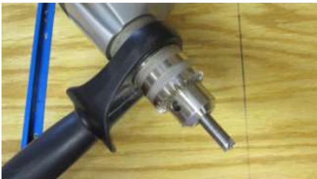
186. The spot weld removal bit seems to work best in drilling the adjacent holes but this process was not easy.
