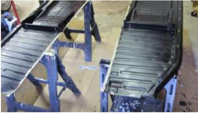
144. The first coat of POR15 completed for both pans.
