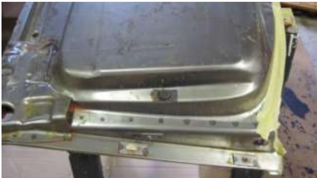
142. I masked off the area, with masking tape, so paint will not get on the areas to be welded.
