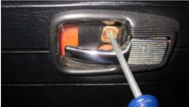
61. With a Phillips screwdriver remove the small screw holding the handle in place.
