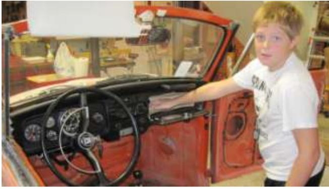
68. Begin removal of the dash off, by emptying the pocket. Then remove the pocket door, ash tray, and all knobs including the radio and fresh air vent knobs. Note: In 2007, I added an accessories gauge panel, this has to be removed before the dash would come off.
