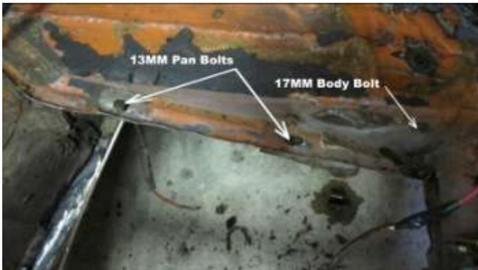
53. Remove body bolts with a 17MM socket. The 13MM pan bolts were removed earlier.
