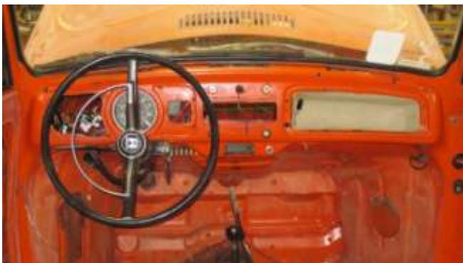
79. View of near empty dash from inside the car. The remaining items will have to be taped up for painting. Note: I had to re-install the light switch button, to drive to the welder once the floor pans are installed.
