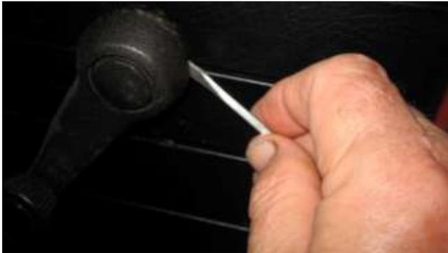
62. With a small screwdriver pry off the plastic portion of the door handle.
