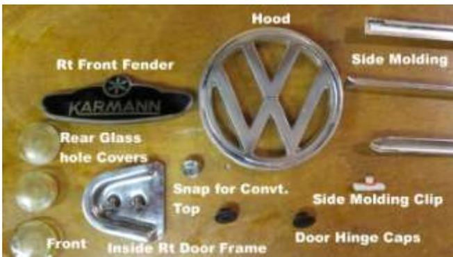
67. Parts removed for the left side and hood are shown at the left. Clean them up with WD40 and dry and label "Right Side Molding" prior to storing in the bag. Then repeat this process for the left side molding.
