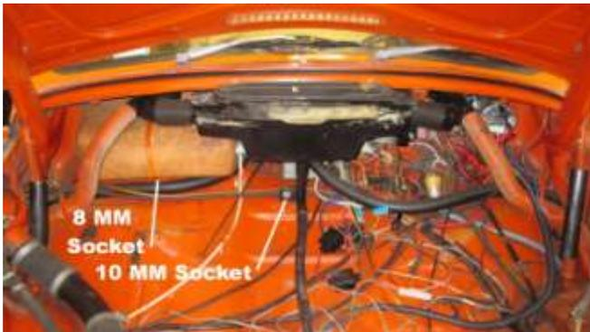
70. Remove the pocket strap with a 8MM socket and then move the pocket out of the way. Note: You do not need to remove the hood latch at this time, since the pocket will be re-installed after all of the dash screws are removed.
