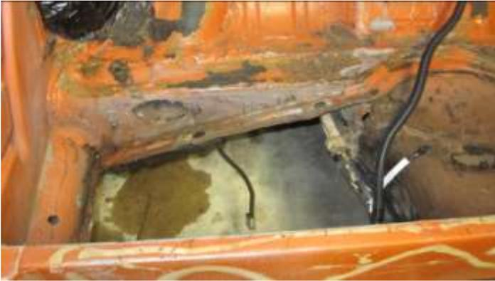
52. Remove remaining passenger side floor pan flange and any remaining portion on floor pan gasket and sand down the heater channel and body portions that connect to the pan. Remove any items in the trunk and perform general cleanup.
