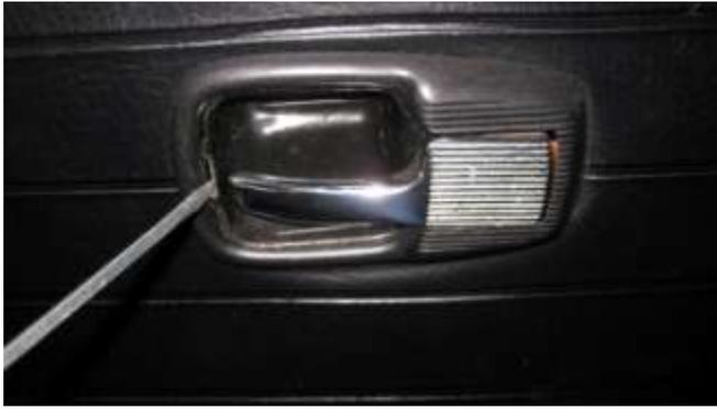
60. With a small screwdriver pry off the inside door handle cap as shown.
