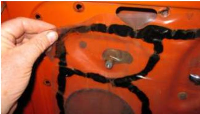
65. Remove the plastic cover between the door and the door panel. Clean off as much of the old sealer as possible.
