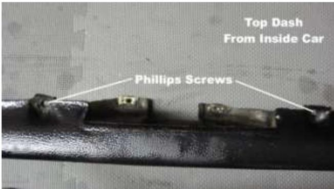
77. Dash blow-up view of the 2 top screws from inside the car.
