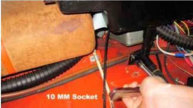
69. Remove the fresh air vent by removing the screws at the top with a screwdriver and the bolt, as shown with a 10MM socket.
