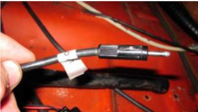
74. Remove the antenna wire to the radio and then remove the radio.
