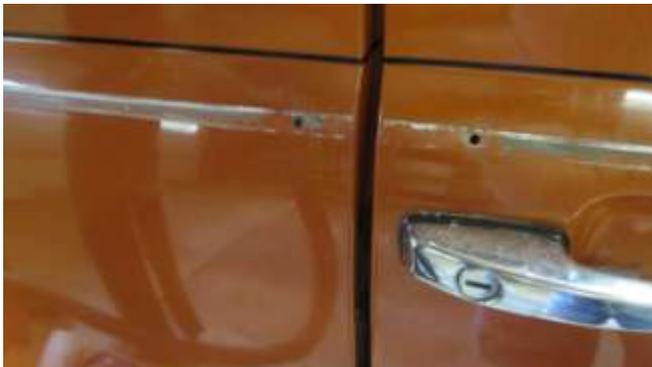
66. With a small screwdriver or small wooden stick, gently remove the side moldings.
