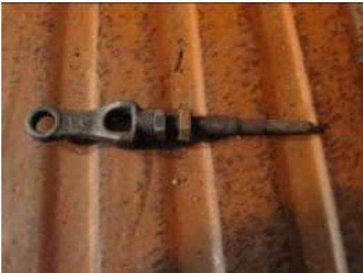
40. Remove the brake rod connector by pulling it straight out.
