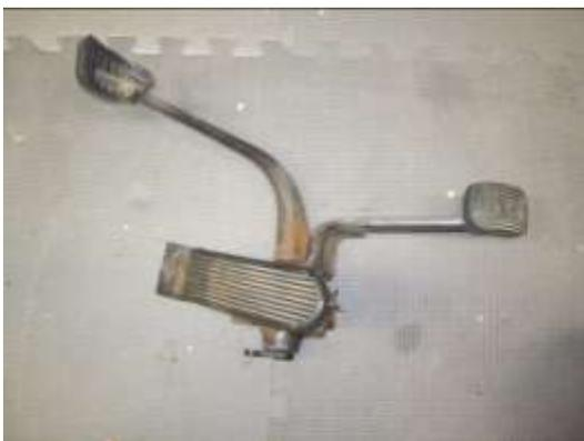
45. Remove the entire pedal cluster assembly and clean with paint thinner and store in a bag with all bolts and brake clip. You can paint this later as necessary.
