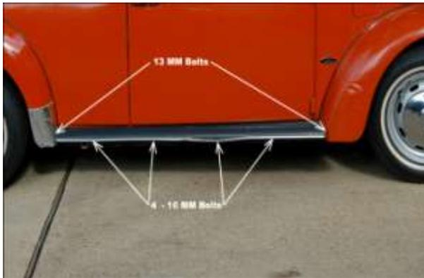
16. For the Running Board there is a 13mm bolt (M8x1.25x20mm) and nut at each fender and four 10mm bolts (M6x1.0x15mm) along the length of the running board as shown.
