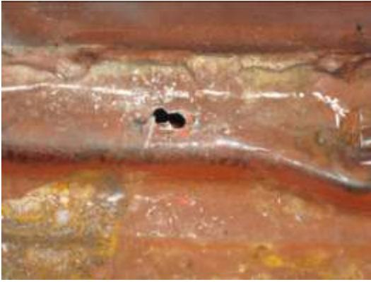
26. Drill two holes close together and wallow them out to allow the saw blade to enter.
