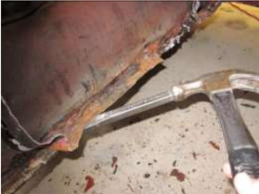
31. Use a chisel and hammer to break the welds loose as shown. This is a slow process, take your time and do it right.
