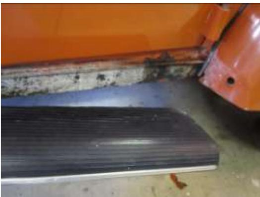
17. Remove the fender bolts and loosen the 4 side bolts and the running board should lift up and out as shown.
