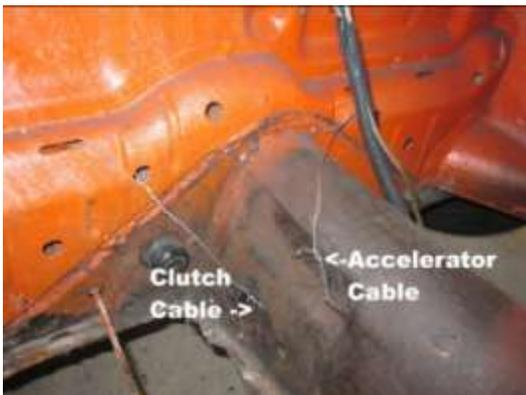
44. Tie the clutch cable out of the way with a string or wire as shown. Check to see if either the clutch or accelerator cable needs to be replaced.
