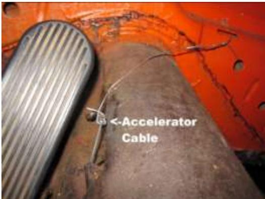
43. Tie the accelerator cable out of the way with a string or wire as shown.
