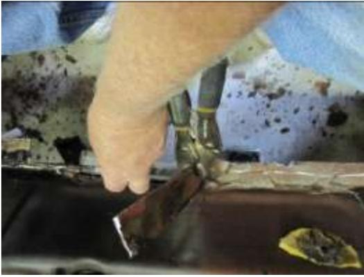
30. Start ripping up the remaining portion of the floor pan.
