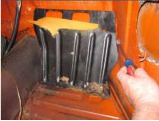
22. Remove the front kick plate on the passenger side with a screwdriver.
