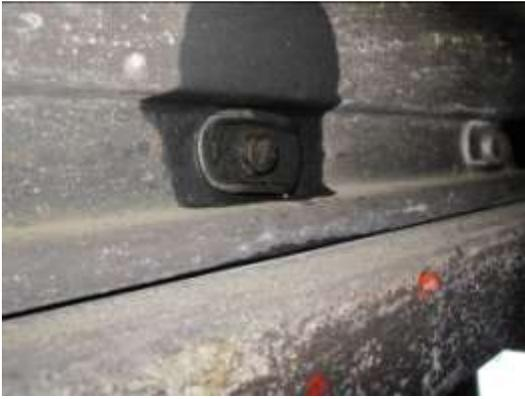
18. For the floor pan use a 13mm socket and remove the 9 bolts under the car as shown. There are 2 more floor pan bolts on each side up front that will be removed later.
