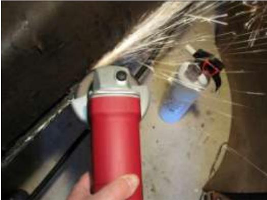
51. Use angle grinder to clean up the welds. Wear goggles, face protection and a long sleeve shirt and have a fire extinguisher close by and make sure no flammables are nearby. Please be careful.
