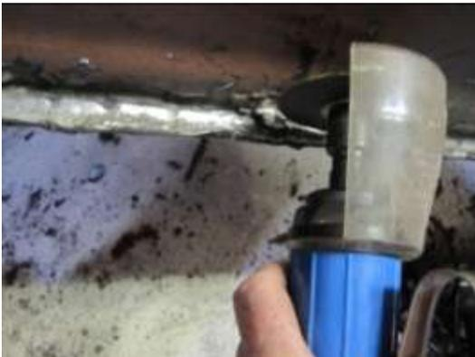
32. Use a cut-off saw to grind the welds off. This is a also a slow process so wait and use a die grinder later.
