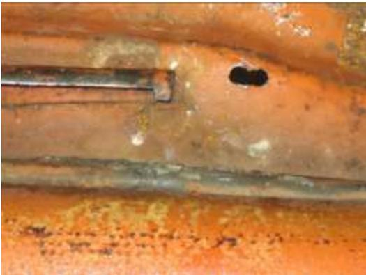
48. Drill starter holes for the saw blade and cut out the driver side pan using the same procedure utilized on the passenger side pan, being very careful around the brake lines and electrical cables.
