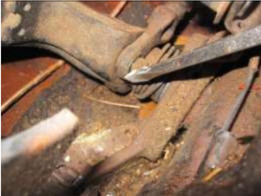
39. Remove the clip on the brake rod connector, with a screwdriver.
