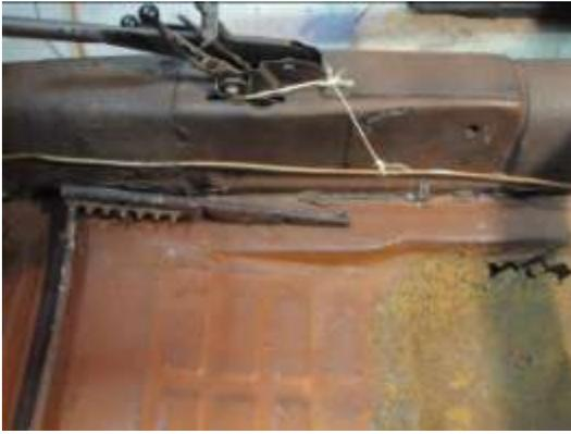
46. Tie the brake line out of the way.
