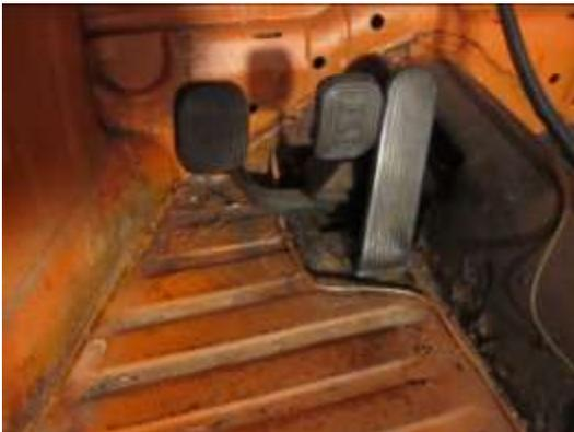
36. Move to the driver side, which requires removing the pedal cluster and protecting the brake lines and the electrical cables.
