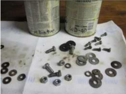
19. Clean the bolts and washers with mineral spirits and then with WD-40. Then dry them off. Discard the rubber washers that mount between the fenders and the running board, buy new ones.
