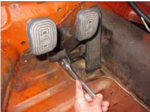
37. Remove the front (M10x1.5x30mm) bolt of the pedal cluster with a 17 mm socket.
