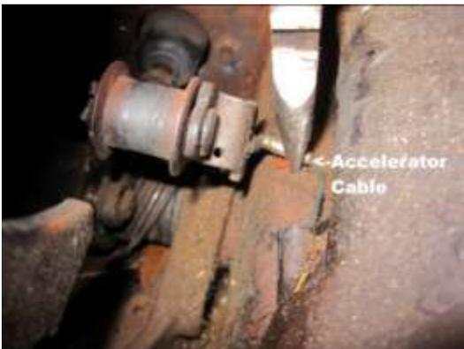
41. Remove the accelerator cable with pliers.
