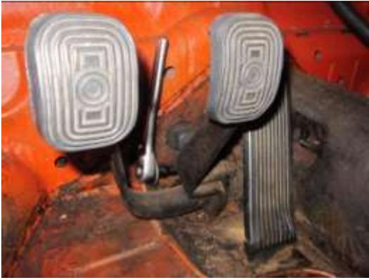
38. Remove the rear bolt of the pedal cluster with a 17 mm socket.
