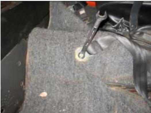
6. Remove all seat belt connections. Use a 16mm wrench to remove all floor connections including the connection under the rear seat. Use a 18mm wrench for the window sill connector and label each seat belt as shown below.
