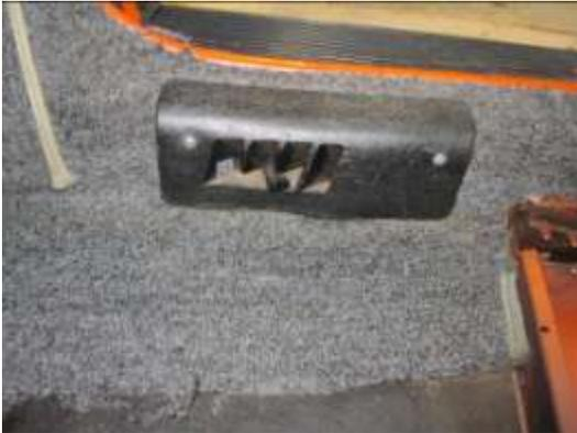
8. Remove the heater ducts with a Phillips screw driver.
