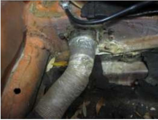
7. Remove the heater tubes connectors with 10mm wrench. This is not an original part. I will try to restore this to original with the factory bakelite parts.
