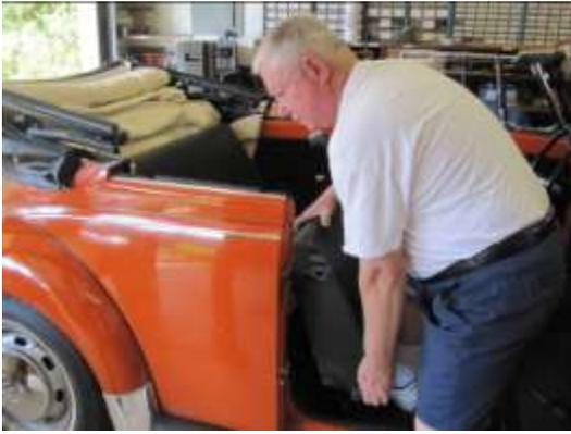
4. Remove the rear seat bottom by pulling the seat up and then pull out on the rear seat.
