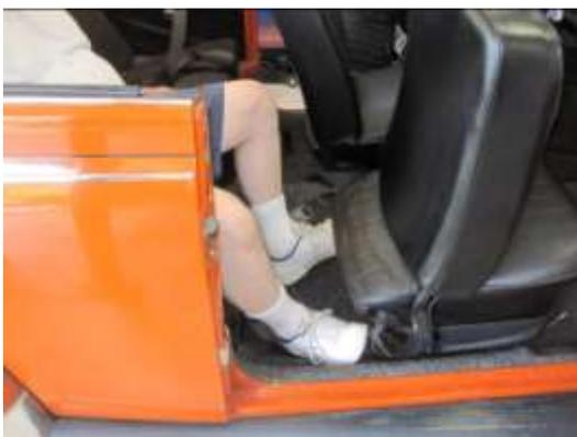
2. You may need someone in the back seat pushing on the seat bottom with their feet, as shown, while someone else is holding down the seat adjustment lever.
