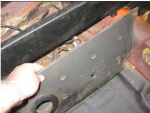
10. Remove the two kick-plates under the rear seat.
