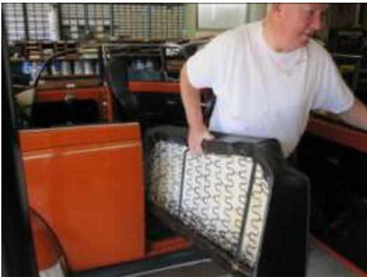
5. Use a 17mm wrench to remove the two pivot bolts on the rear seat back to remove the back of the rear seat.
