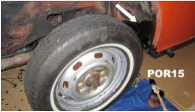
319. Apply one coat of POR15 on all fender wells, again wear long sleeves and gloves as this gets messy and once the POR15 dries it is very hard to get off.
