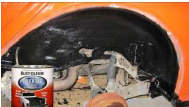
322. The next day paint the wheel well openings with Rust-Oleum Truck Bed Liner material to fight future rust.
