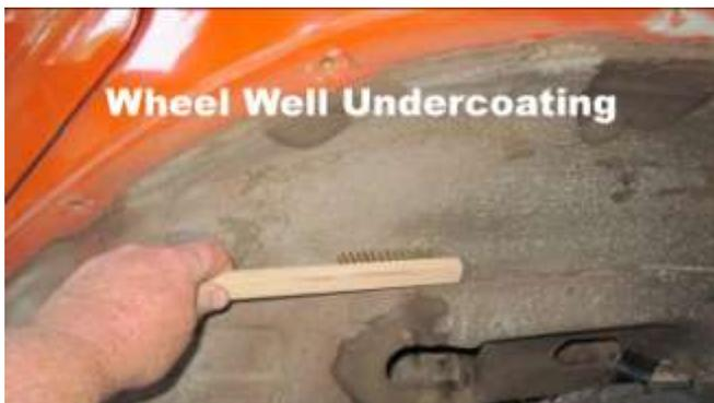
315. Back car outside and wire brush all four wheel wells and suspension to scrape any loose grease or undercoating off.
