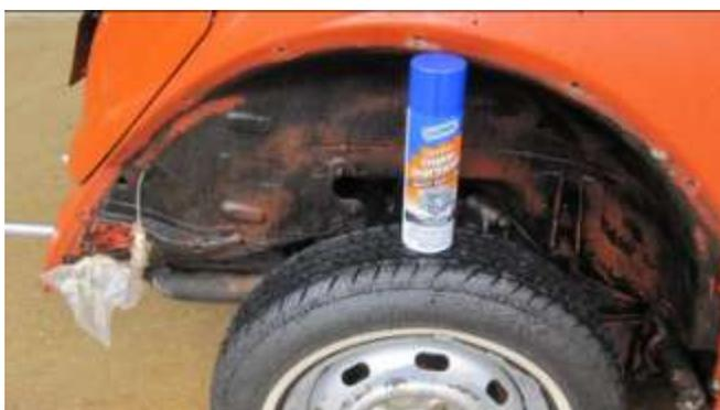
317. Spray one can of Gunk on the rear two fender wells and suspension including under the engine.
