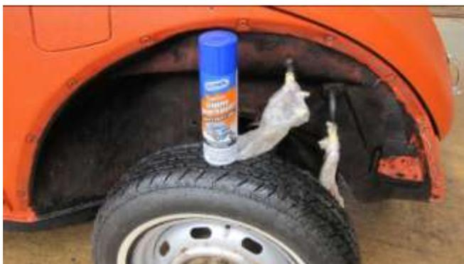
316. Spray one can of Gunk on the front two fender wells and suspension.
