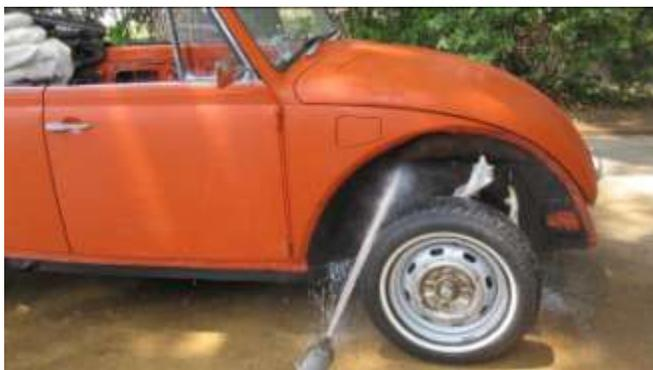
318. Wait 15 minutes and wash down all fender wells, suspension, and the under carriage area. Let air dry and move car inside to air dry overnight.
