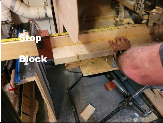
4. Close up of my temporary stop block assembly.
