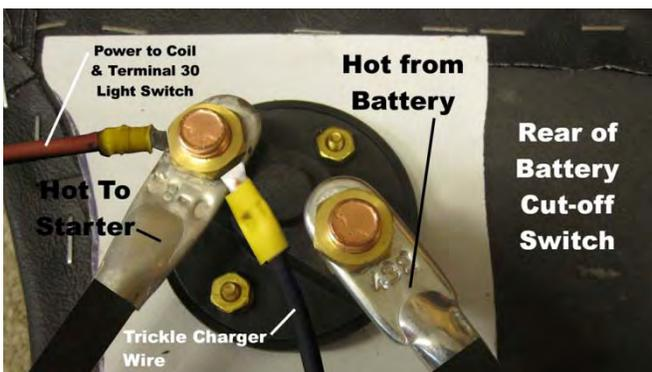
8. A new positive cable was purchased and it was cut off to about 12" and a new terminal was solders on the cut end. The wires were then connected as shown.
