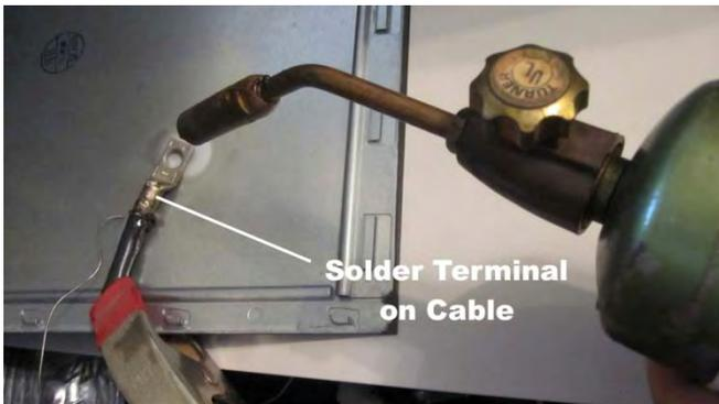
7. The rear of the car was covered up with an old blanket and metal plates were used as shields as shown and the terminal was soldered to the wire.
