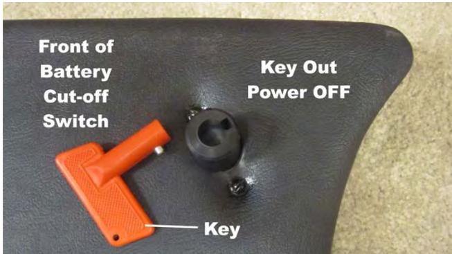
3. When the key is removed the power does not go to the car starter or voltage regulator or terminal 30 of the light switch therefore no power to the starter key.
