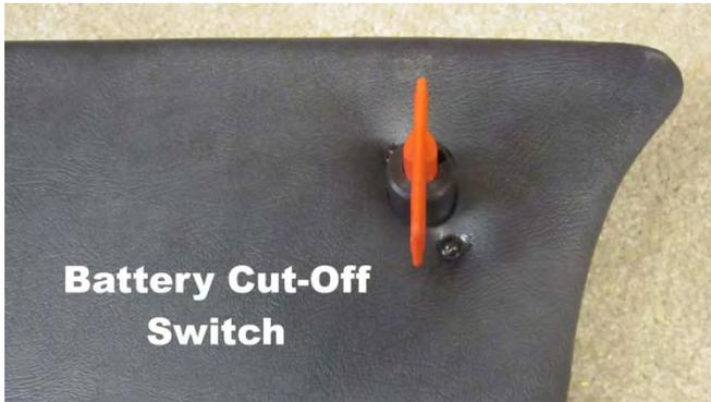
1. I wanted to make life easier and every time I needed to disconnect the battery I had to take up the back seat out and disconnect the positive wire from the battery even when I towed the car the battery had to be disconnected so that the key could be left in the ON position when towing, so I installed the battery cut-off switch as shown.
